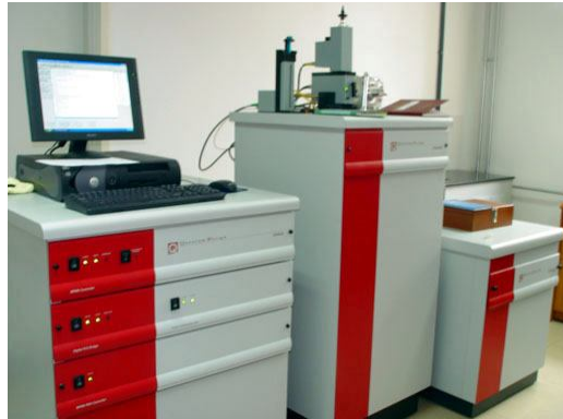
Figure 2.43: A Quantum Design MPMS XL SQUID magnetometer at the University of Manchester (Taken from [74]).
