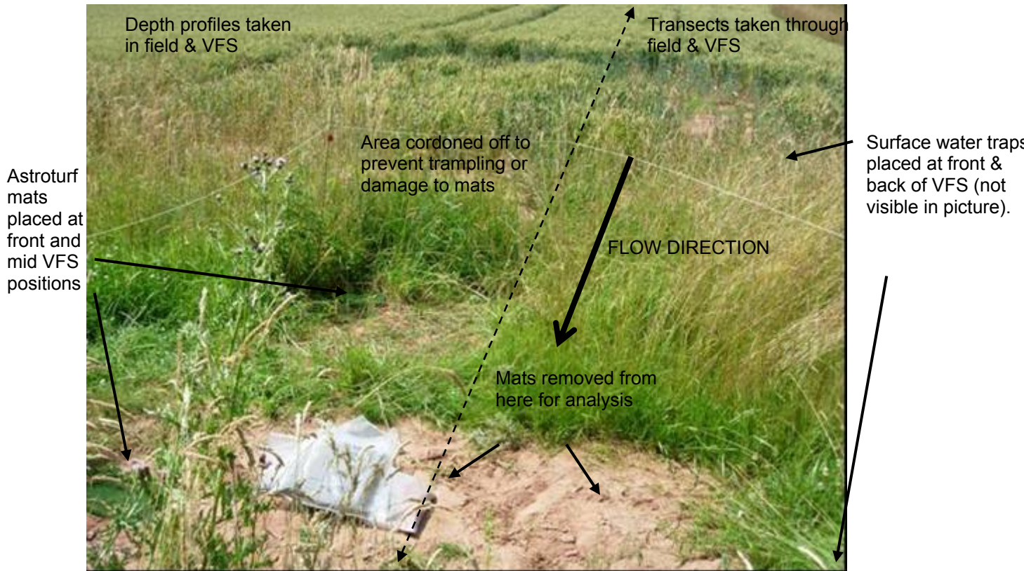
Figure 5.13 Typical field set up (Site 7). Astroturf mats, surface water traps, 120 mm depth profiles and transects of 20 mm sediment cores were used at each site.
