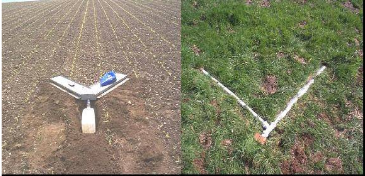
Figure 5.12 Metal (left) and plastic (right) surface water traps. Each design consists of two arms at a 90° angle facing upslope and a collection vessel. Water flows into the upslope edge of the arms and is channelled into a plastic container for collection.
