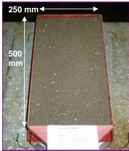
Figure 4.4 Experimental tray packed with soil prior to simulated rainfall.
