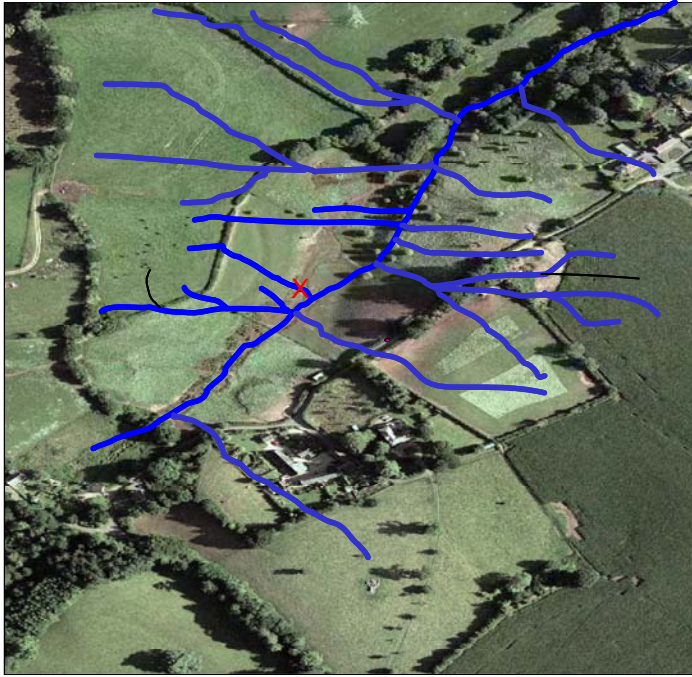
Figure 5.9 Aerial photograph of an example site with lines representing the flowpath network of the subcatchment. X marks the monitoring site.
