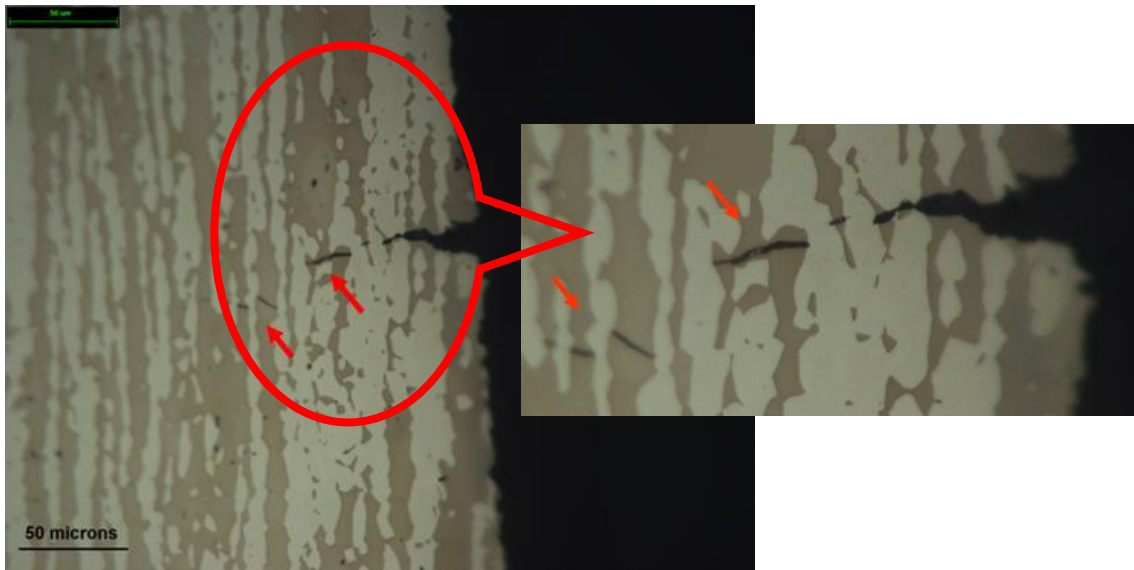
Figure 5.76: Optical micrograph of internal microcrack on failed cross section of super DSS SAF 2507 precharged at -1250 mV for 2 weeks
