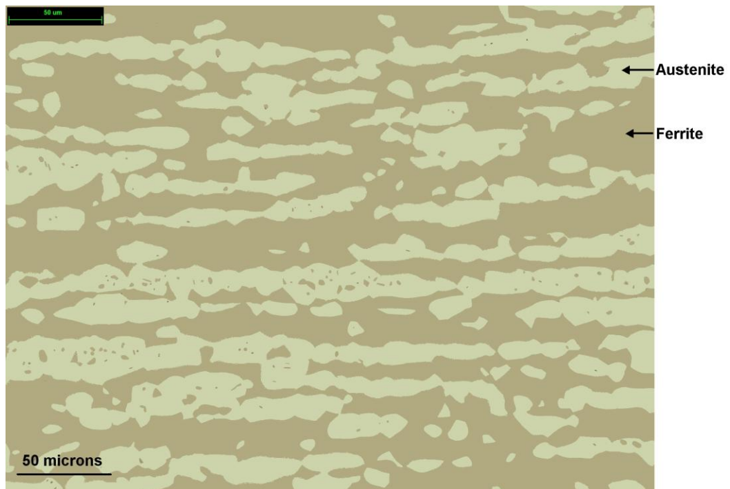
Figure 5.2: Optical micrograph of the longitudinal section of SDSS Ferralium 255 etched by 10M NaOH solution
