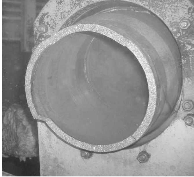
Figure 2.10: Fracture surface of in board side of parted subsea hub 16
