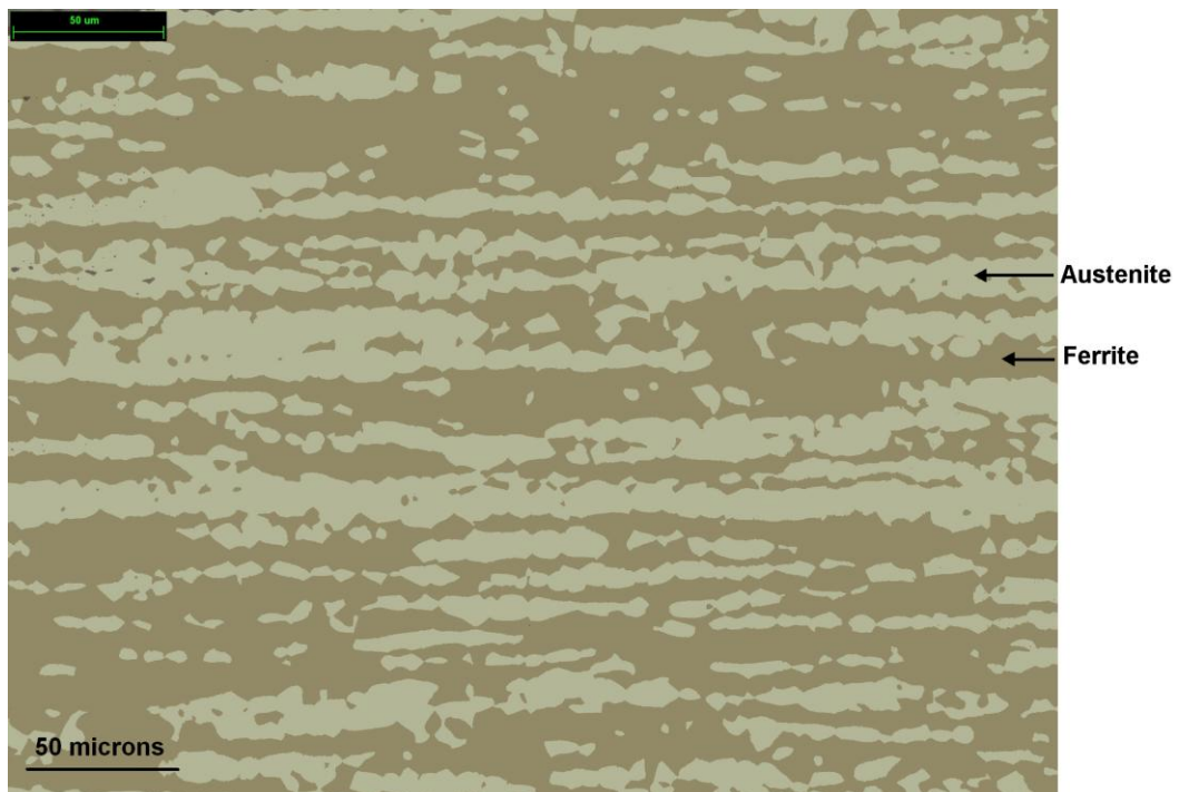
Figure 5.4 Optical micrograph of the longitudinal section of SDSS SAF 2507 etched by 10M NaOH solution
