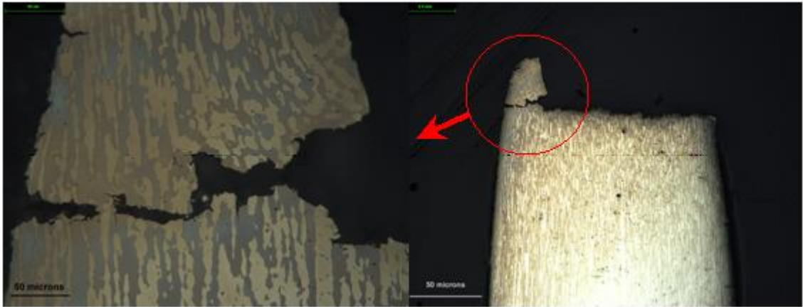
Figure 5.72: Optical micrograph of crack profile on failed cross section of super DSS SAF 2507 precharged at -1250 mV for 2 weeks
