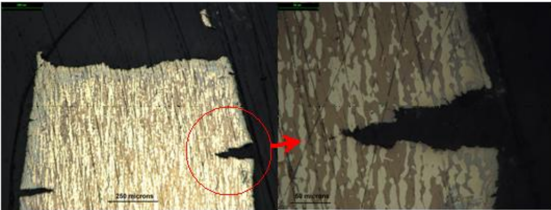
Figure 5.73: Optical micrograph of crack profile on failed cross section of super DSS Ferralium 255 precharged at -1250 mV for 2 weeks
