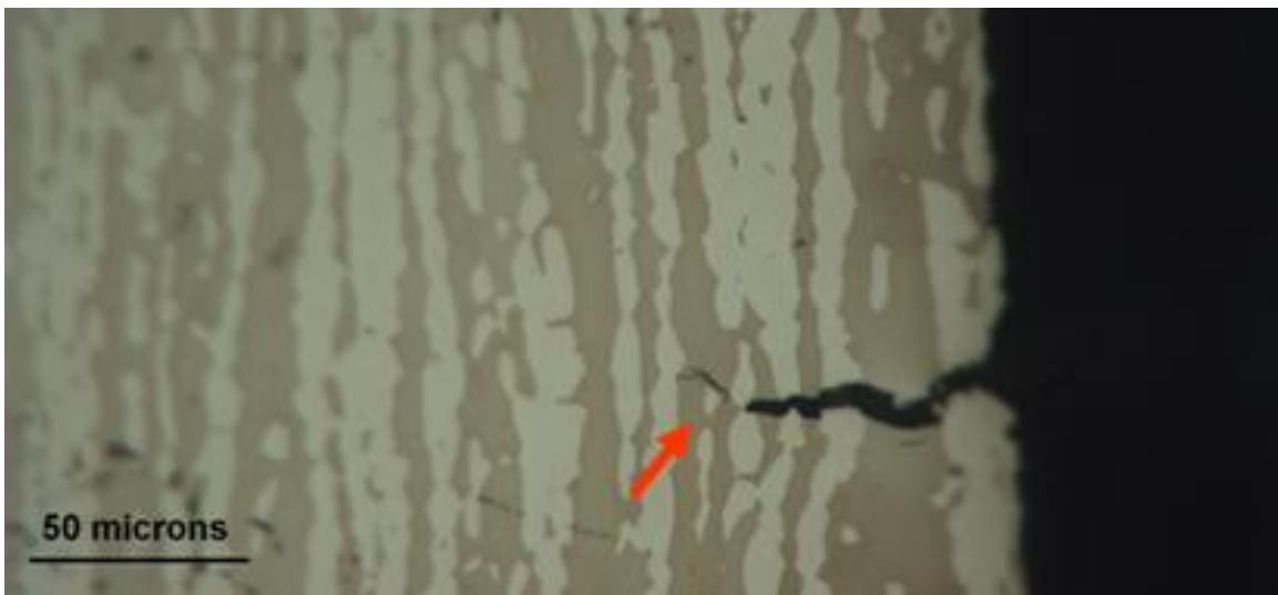
Figure 5.75: Optical micrograph of internal microcrack on failed cross section of super DSS SAF 2507 precharged at -1250 mV for 2 weeks
