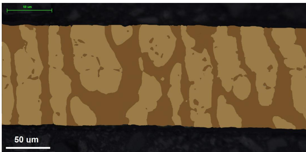
Figure 5.95: Cross section of 100 \mu\text{m} thick membrane used in the galvanostatic test for super DSS SAF 2507 showing the direction of the colonies of the austenite grains
