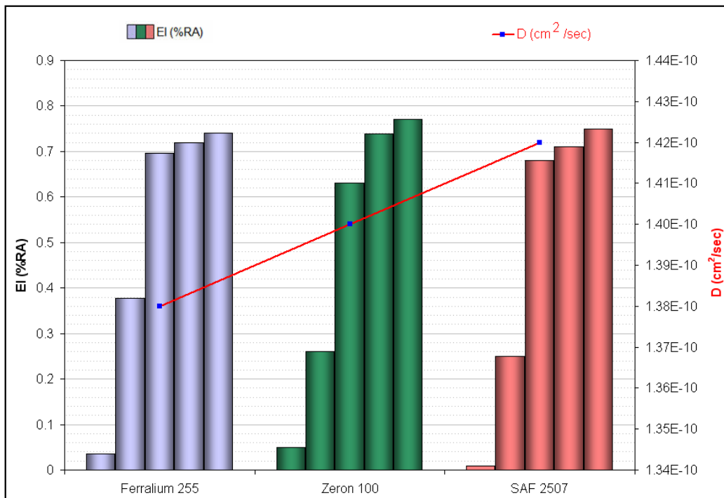
Figure 7.9: Comparison of hydrogen diffusion coefficient and the mean embrittlement index (%RA) for the three alloys
