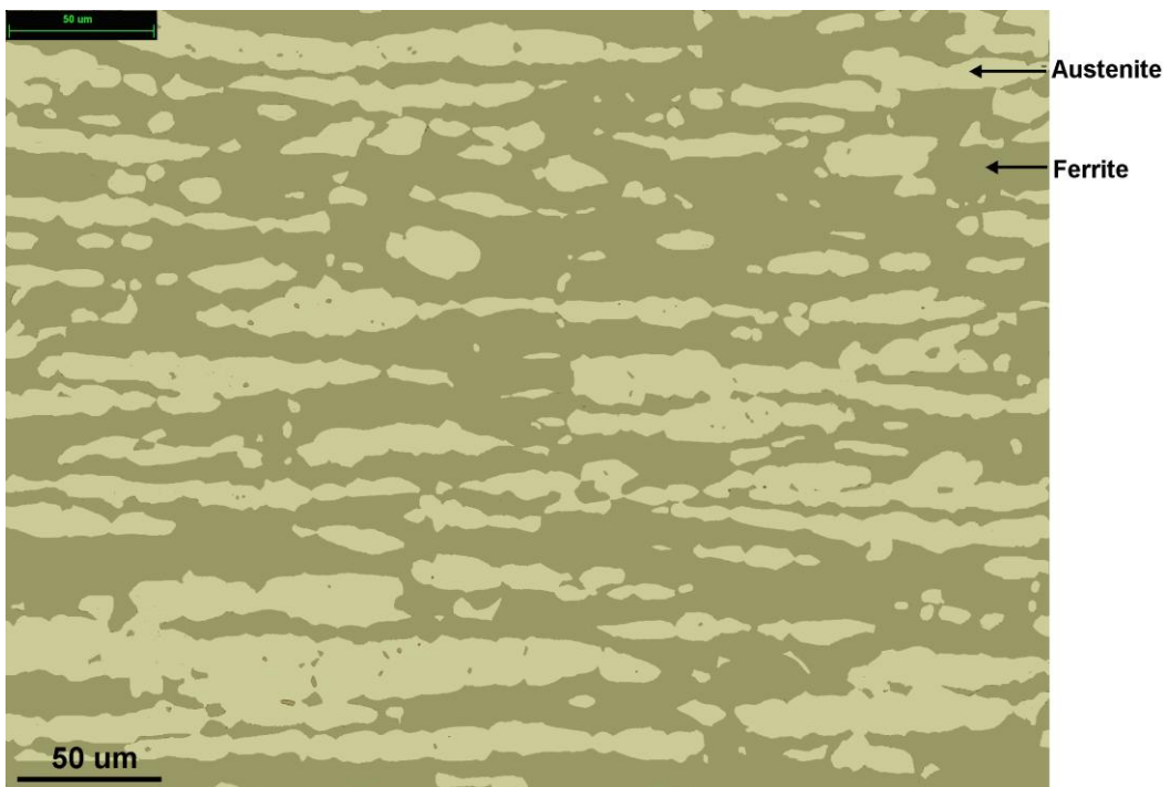
Figure 5.6: Optical micrograph of the longitudinal section of SDSS Zeron 100 etched by 10M NaOH solution
