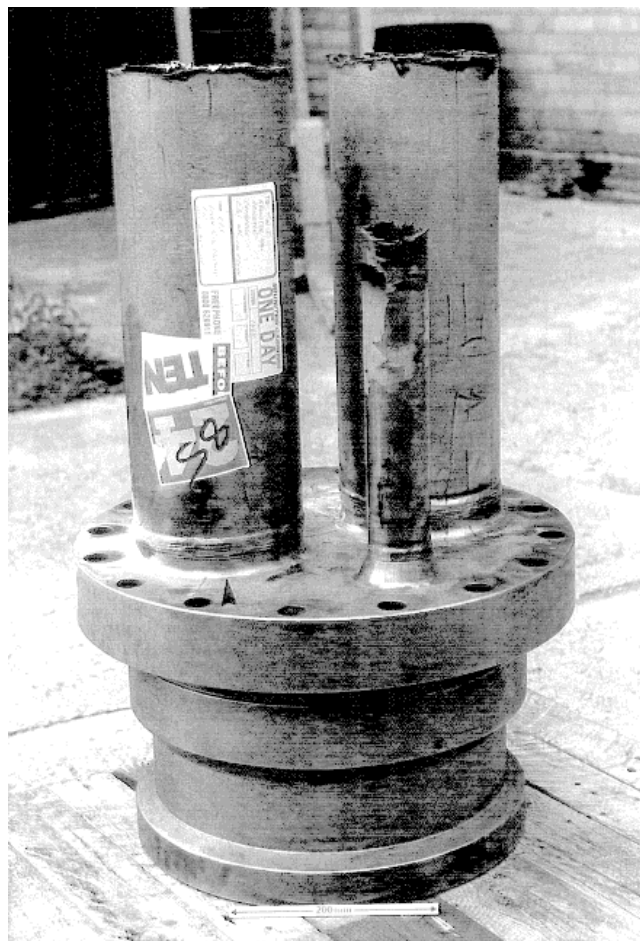
Figure 2.8 : Super duplex stainless steel hub forging with welded pipe connections 15
