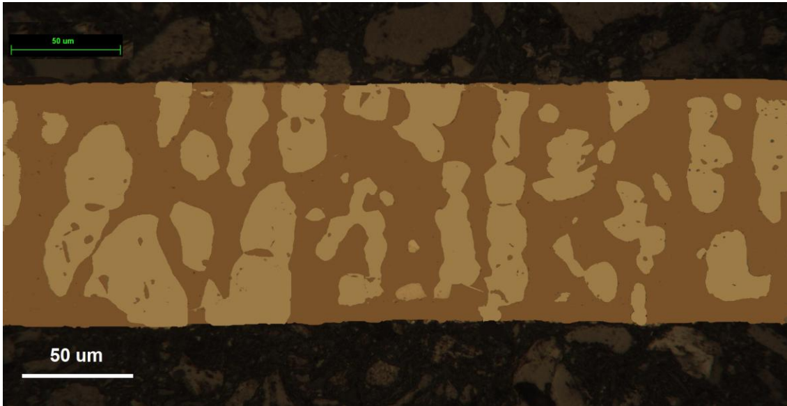
Figure 5.91: Cross section of 100 μm thick membrane used in the galvanostatic test for super DSS Ferralium 255 showing the orientation of the colonies of the austenite grains
