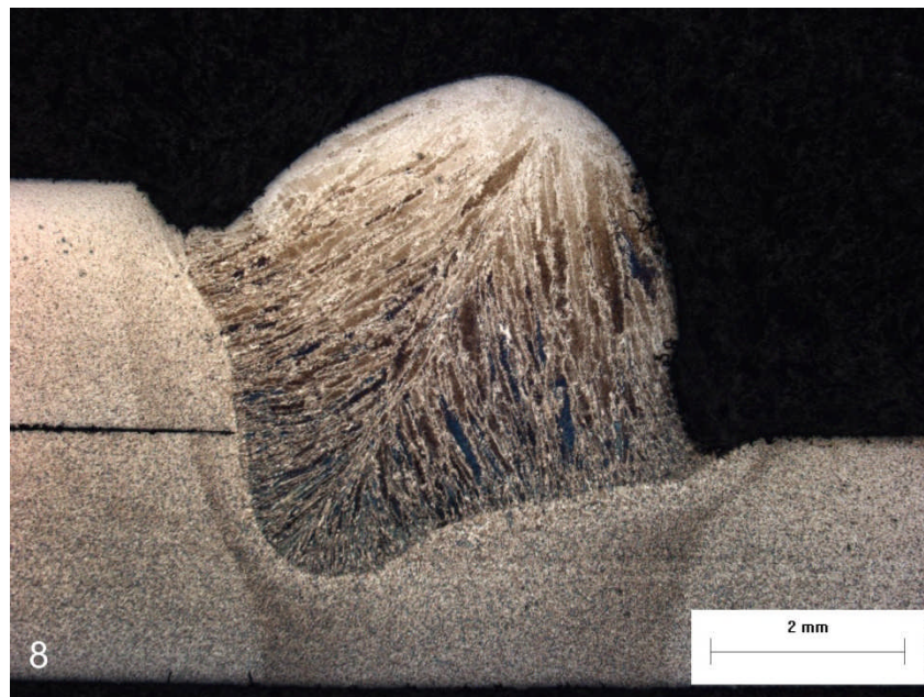
Figure 6.52 Macrosection for a Dual-Spot Nd:YAG Hybrid Weld Made at 4.0-m/min on 2.4-mm Sheet
