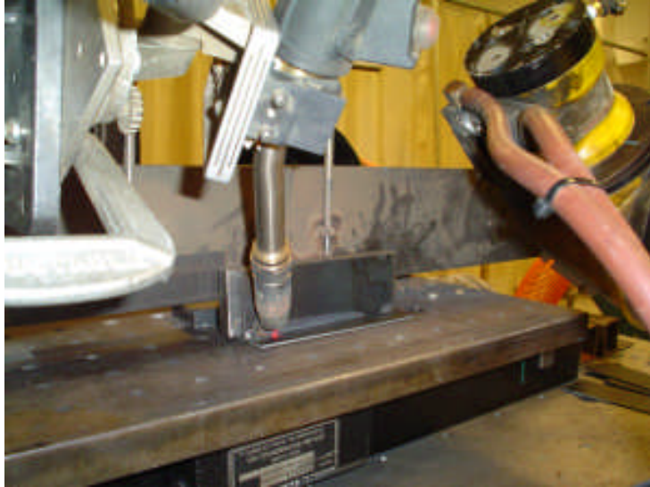
Figure 4.15 Laser Spot Alignment Using a Low-Power Visible Red He-Ne Laser
