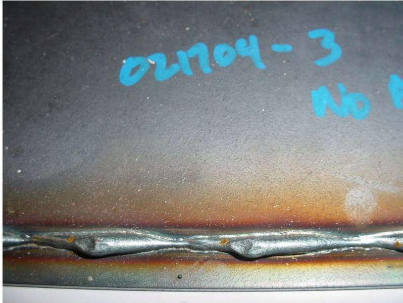
Figure 6.47 GMAW-P Fillet Weld on a Lap Joint
