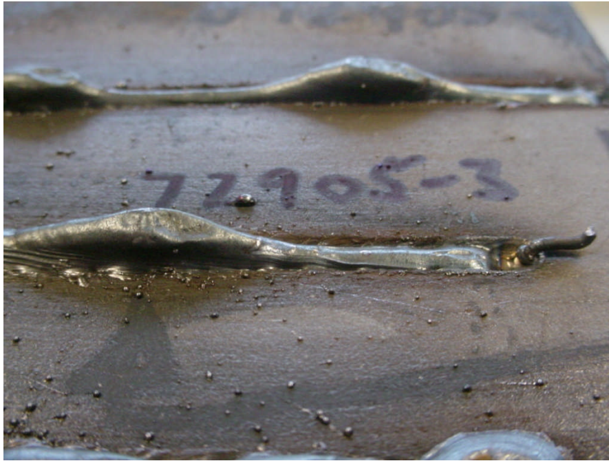
Figure 6.78 Side View of GMAW-P BOP Humping and Weld Pool Cavity for Specimen 72905-3 WFS 15.2 m/min, TS 2.5 m/min, 225 A, 35 V, 16-mm CTWD, 5-mm Plate
