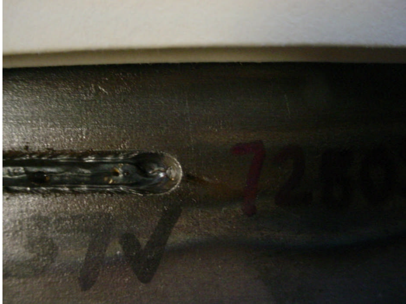
Figure 6.65 Plan View of GMAW-P Weld Pool Cavity for Specimen 72805a WFS 15.2 m/min, TS 2.5 m/min, 225 A, 37 V, 19-mm CTWD
