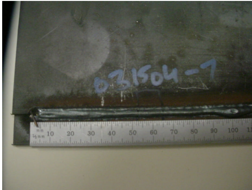
Figure 6.49 36-mm-Long Weld Pool with 3-mm Bead Width (12:1) using Single-Spot 4-kW Nd:YAG/GMAW-P Hybrid on a Lap Joint
