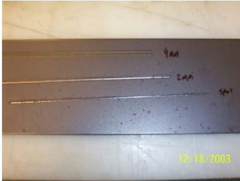
Figure 6.37 Spot and Scanned Nd:YAG Laser Profiles in BOP Form
