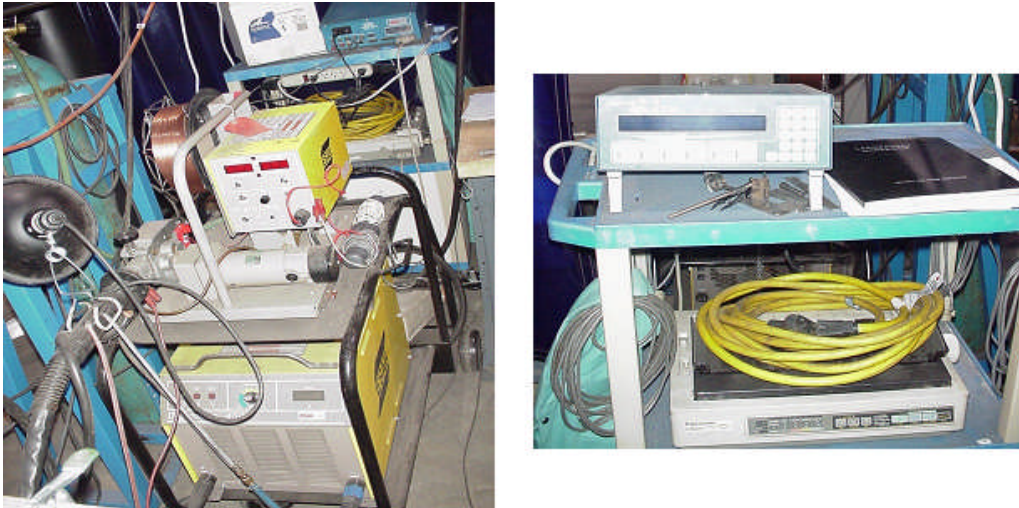
Figure 4.2 Welding Power Supply and Wire Feeder (left), Data Acquisition System (right) used for Gap Weldability Testing
