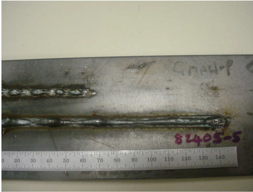
Figure 6.90 Plan View of GMAW-P BOP Humping for Specimen 82405-5 WFS 15.2 m/min, TS 3.0 m/min, 225 A, 34 V, 16-mm CTWD, 1.6-mm Sheet (lower bead) and for Specimen 82405-4 WFS 15.2 m/min, TS 3.0 m/min, 225 A, 31 V, 16-mm CTWD, 1.6-mm Sheet (upper bead)
