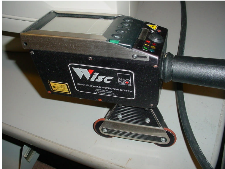
Figure 4.26 WISC Laser Profilometer
