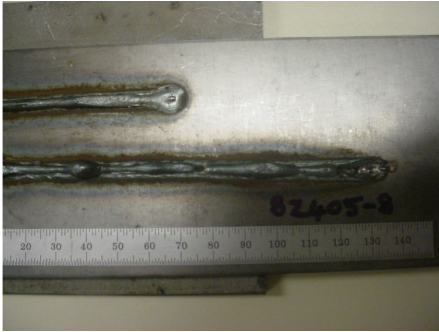
Figure 6.95 Plan View of GMAW-P BOP Humping for Specimen 82405-8 WFS 15.2 m/min, TS 3.0 m/min, 225 A, 34 V, 16-mm CTWD, 1.6-mm Sheet
