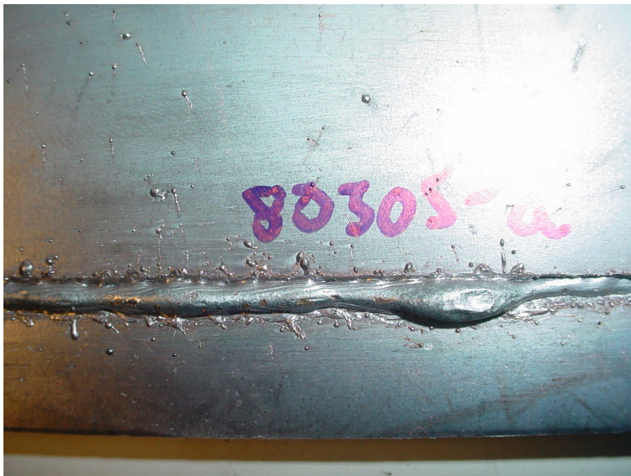
Figure 6.84 Plan View of GMAW-P Fillet Weld Humping in a LapJoint for Specimen 80305a WFS 15.2 m/min, TS 3.0 m/min, 225 A, 34 V, 16-mm CTWD, 1.6-mm Sheet
