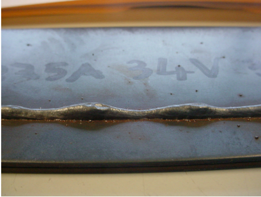
Figure 6.83 Side View of GMAW-P BOP Humping for Specimen 80205b WFS 15.2 m/min, TS 2.5 m/min, 225 A, 34 V, 19-mm CTWD,
