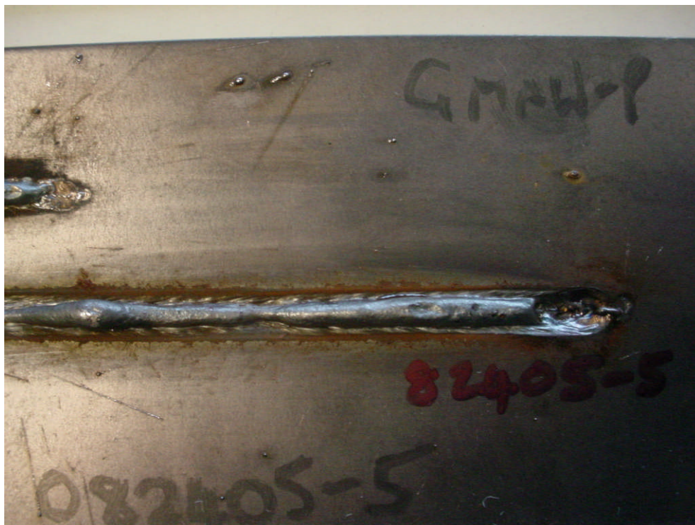
Figure 6.89 Plan View of GMAW-P BOP Humping for Specimen 82405-5 WFS 15.2 m/min, TS 3.0 m/min, 225 A, 34 V, 16-mm CTWD, 1.6-mm Sheet
