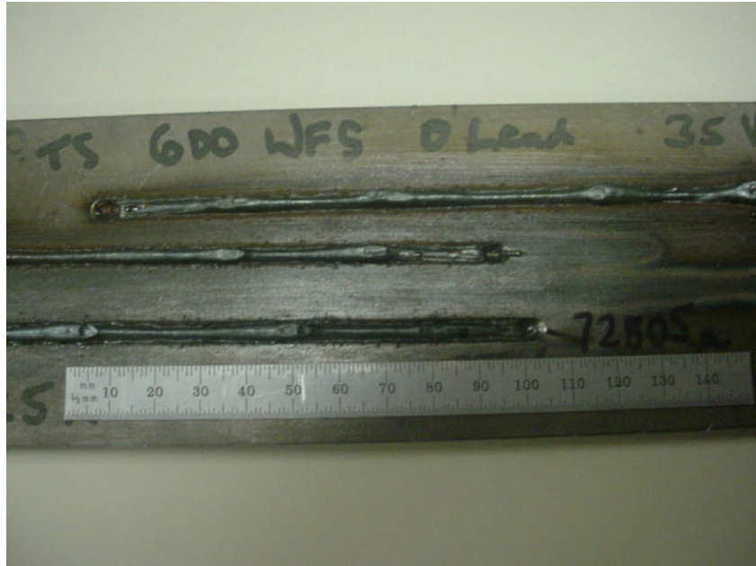
Figure 6.67 Plan View of GMAW-P BOP Humping for Specimen 72805a WFS 15.2 m/min, TS 2.5 m/min, 225 A, 37 V, 19-mm CTWD, 5-mm Plate
