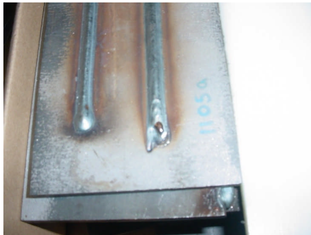
Figure 7.5 Wetting of the Weld Toe Using a Single Laser Spot (Seen at Left of the Right-Hand Weld Bead)
