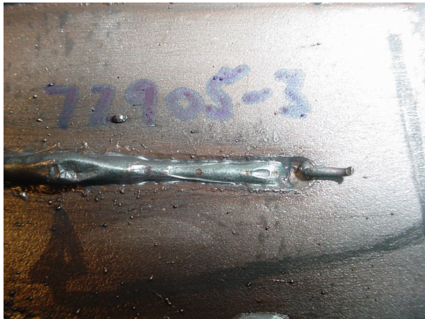
Figure 6.77 Plan View of GMAW-P BOP Humping and Weld Pool Cavity for Specimen 72905-3 WFS 15.2 m/min, TS 2.5 m/min, 225 A, 35 V, 16-mm CTWD, 5-mm Plate
