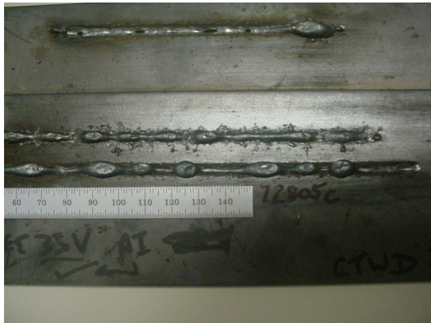
Figure 6.72 Plan View of GMAW-P BOP Humping and Weld Pool Cavity for Specimen 72805c WFS 15.2 m/min, TS 2.5 m/min, 225 A, 31 V, 19-mm CTWD, 2.4-mm Sheet
