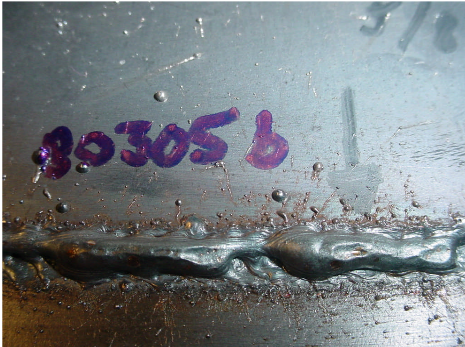
Figure 6.86 Plan View of LBW/GMAW-P Fillet Weld Humping in a Lap Joint for Specimen 80305b with Wire Offset too Much onto the Top Sheet WFS 15.2 m/min, TS 3.0 m/min, 225 A, 34 V, 16-mm CTWD, 1.6-mm Sheet
