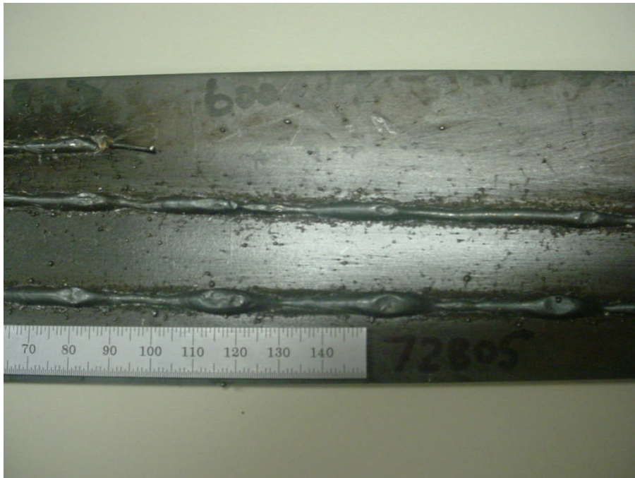
Figure 6.69 Plan View of GMAW-P BOP Humping for Specimen 72805 WFS 15.2 m/min, TS 2.5 m/min, 225 A, 28 V, 19-mm CTWD, 2.4-mm Plate
