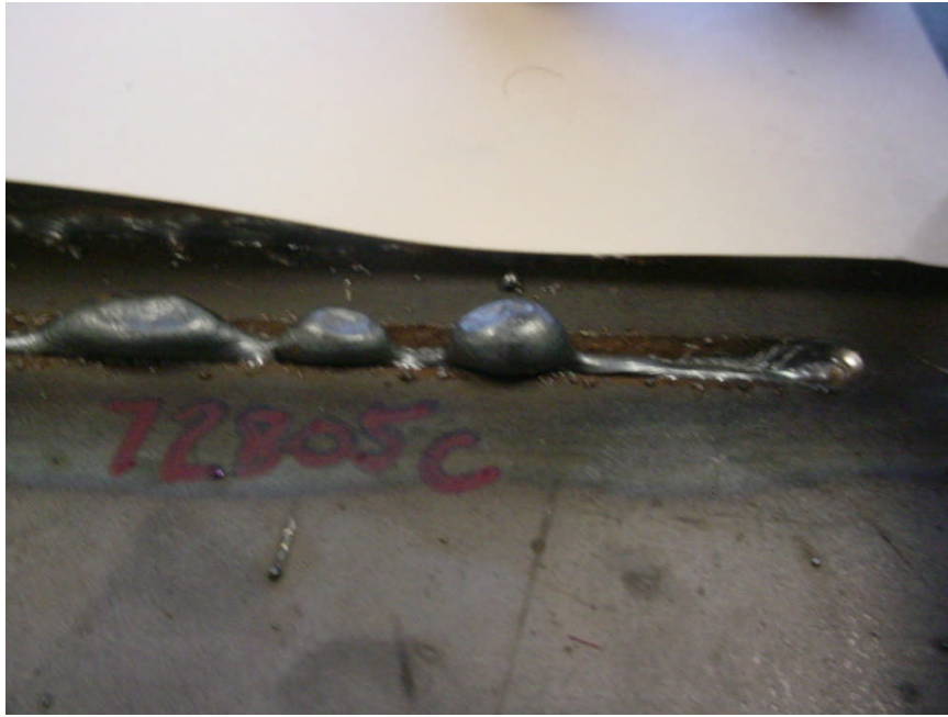
Figure 6.73 Side View of GMAW-P BOP Humping and Weld Pool Cavity for Specimen 72805c WFS 15.2 m/min, TS 2.5 m/min, 225 A, 31 V, 19-mm CTWD, 2.4-mm Sheet
