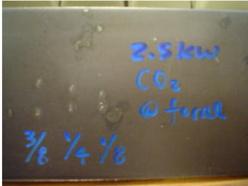
Figure 5.6 Adjustable Beam Distance for CO 2 Laser Split Optics showing 3.2-, 6.4- and 9.5-mm Dual Spot Spacing
