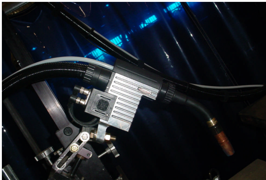
Figure 2.5 Fronius CMT Gun With Integrated Wire Feed Motor for Forward and Reverse Wire Drive
