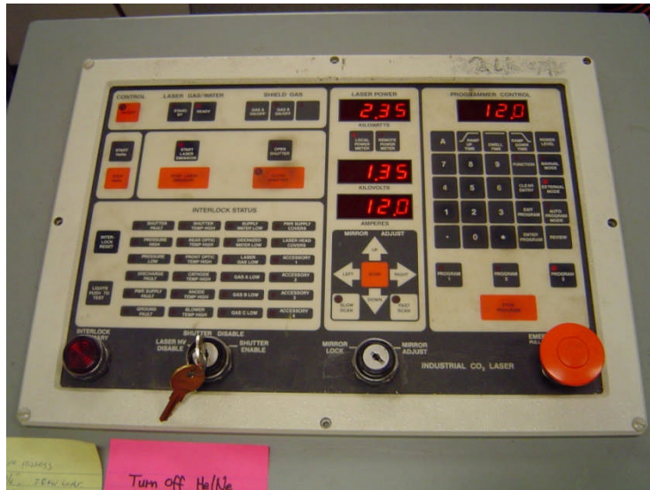
Figure 4.16 Console for Laser Parameter Selection
