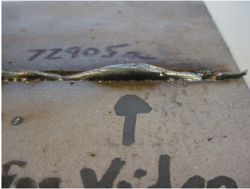
Figure 6.76 Side View of GMAW-P BOP Humping for Specimen 72905a WFS 15.2 m/min, TS 2.5 m/min, 225 A, 33 V, 16-mm CTWD, 5-mm Plate
