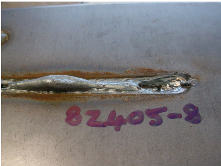
Figure 6.96 Side View of GMAW-P BOP Humping for Specimen 82405-8 WFS 15.2 m/min, TS 3.0 m/min, 225 A, 34 V, 16-mm CTWD, 1.6-mm Sheet
