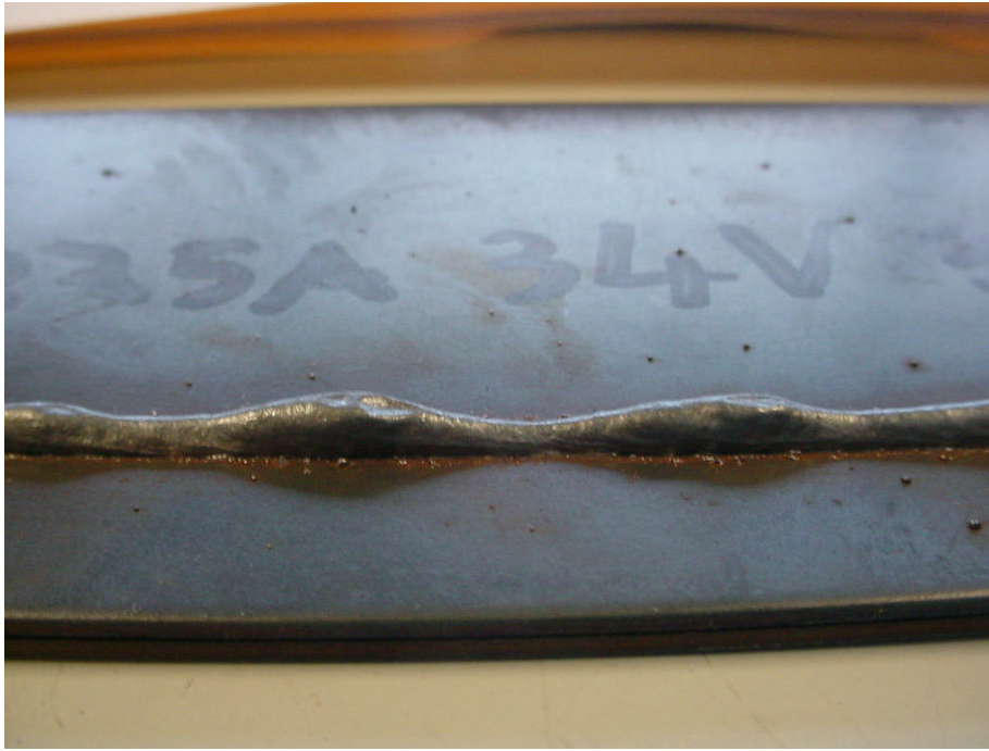
Figure 7.18 Side View of GMAW-P BOP Humping in 1.6-mm Sheet Metal for Specimen 80205b
