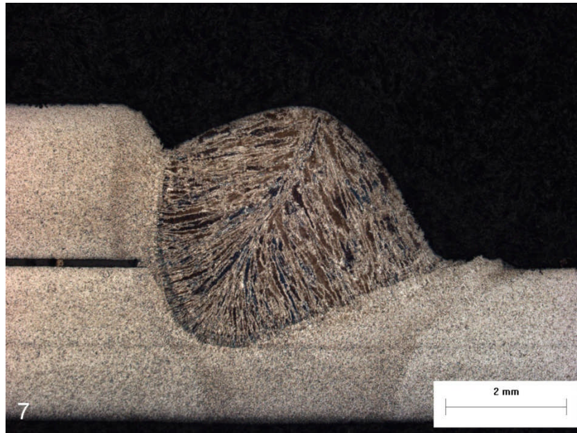
Figure 6.51 Macrosection for Dual-Spot Nd:YAG Hybrid Weld Made at 3.3 m/min on 2.4-mm Sheet
