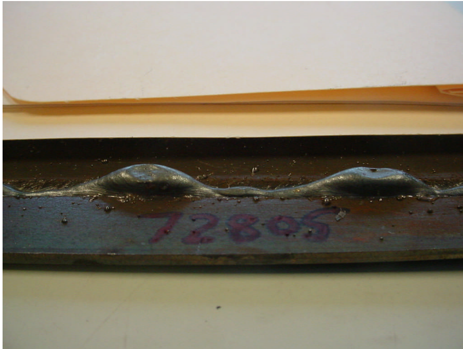
Figure 6.70 Side View of GMAW-P BOP Humping for Specimen 72805 WFS 15.2 m/min, TS 2.5 m/min, 225 A, 28 V, 19-mm CTWD, 2.4-mm Sheet
