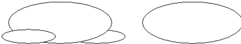
Figure 7.13 Cross-Sectional View - Size and Arrangement of Laser beam Spots (Small Elliptical Spot) Relative to the Arc Weld Pool (Ellipse) at Left, Resulting in Minimum Weld Toe Wetting and Spreading at Right
