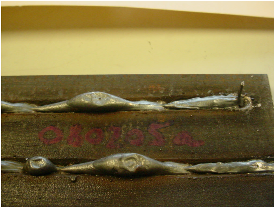
Figure 6.80 Side View GMAW-P BOP Humping and Weld Pool Cavity for Specimen 80205a WFS 15.2 m/min, TS 2.5 m/min, 225 A, 34 V, 19-mm CTWD, 5-mm Plate
