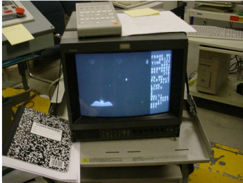
Figure 4.23 Typical Screen Image and Frame Data Using the Kodak Ektapro HS System
