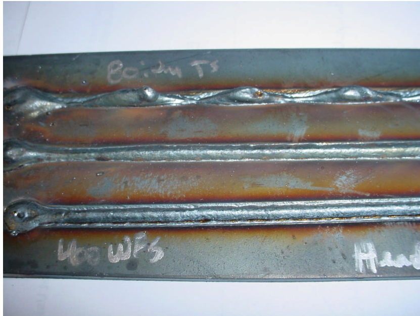
Figure 7.25 Classic Bead Humping (Top Bead) for GMAW-P Suppressed with 1-kW Nd:YAG Laser Energy (Middle and Bottom) (WFS/TS of 5 - BOP Weld) at 2.0-m/min TS
