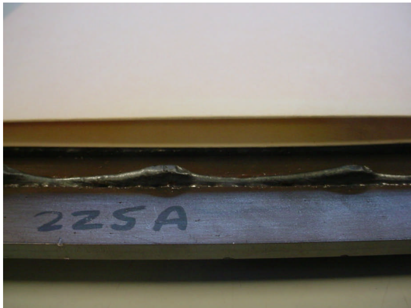
Figure 6.66 Side View of GMAW-P BOP Humping for Specimen 72805a WFS 15.2 m/min, TS 2.5 m/min, 225 A, 37 V, 19-mm CTWD, 5-mm Plate
