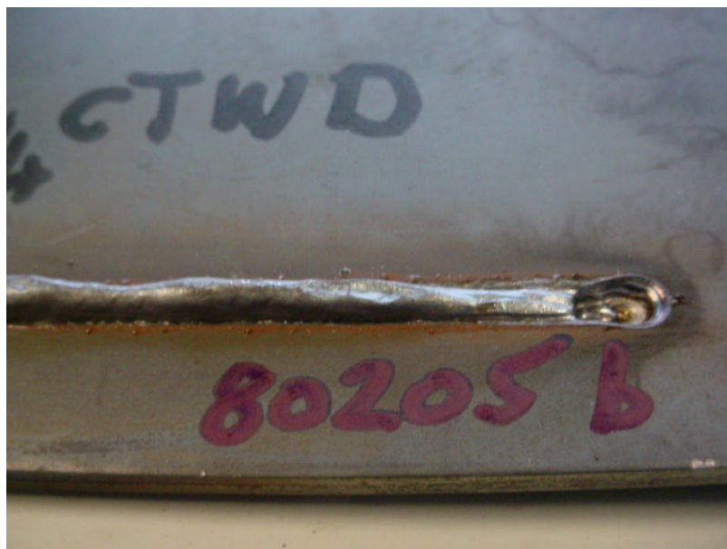
Figure 6.82 Side View of GMAW-P BOP Humping and Weld Pool Cavity for Specimen 80205b WFS 15.2 m/min, TS 2.5 m/min, 225 A, 34 V, 19-mm CTWD, 1.6-mm Sheet
