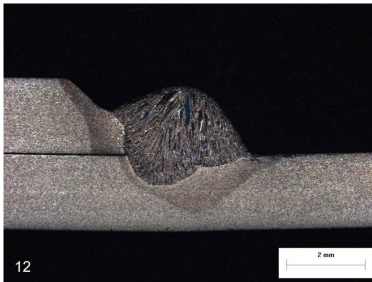
Figure 6.60 Macrosection for a Single-Spot CO 2 LBW/GMAW-P Hybrid Weld Made at 4 m/min on 2-mm Sheet
