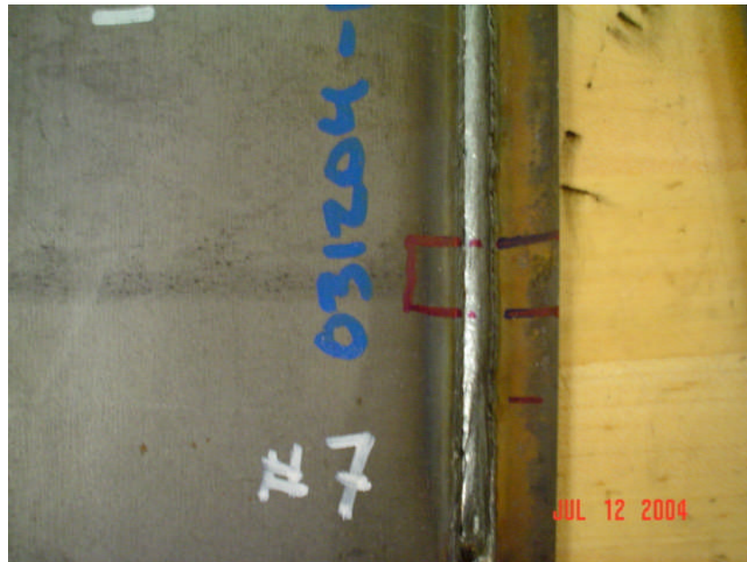
Figure 6.50 Bead Appearance for Dual-Spot Nd:YAG Hybrid Weld made at 3.3 m/min on a Lap-Fillet Joint 2.4-mm Sheet
