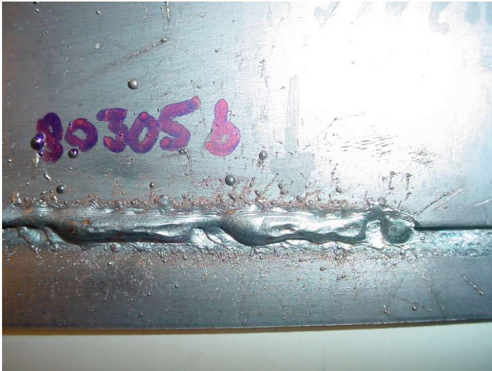
Figure 6.87 Side View of LBW/GMAW-P Fillet Weld Humping in a Lap Joint for Specimen 80305b with Wire Offset too Much onto the Top Sheet WFS 15.2 m/min, TS 3.0 m/min, 225 A, 34 V, 16-mm CTWD, 1.6-mm Sheet
