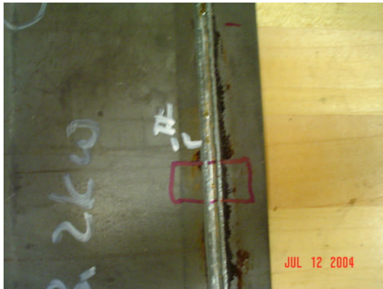
Figure 6.59 Bead Appearance for a Lap-Fillet Joint Made Using Single-Spot CO 2 LBW/GMAW-P Hybrid Welding with 3.25-kW Laser Power at 4-m/min TS on 2-mm Sheet
