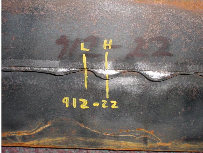
Figure 6.19. Continuous Humping Defect Generated at a 1T Gap on a Joint at a ‘High’ 1.0-m/min TS
