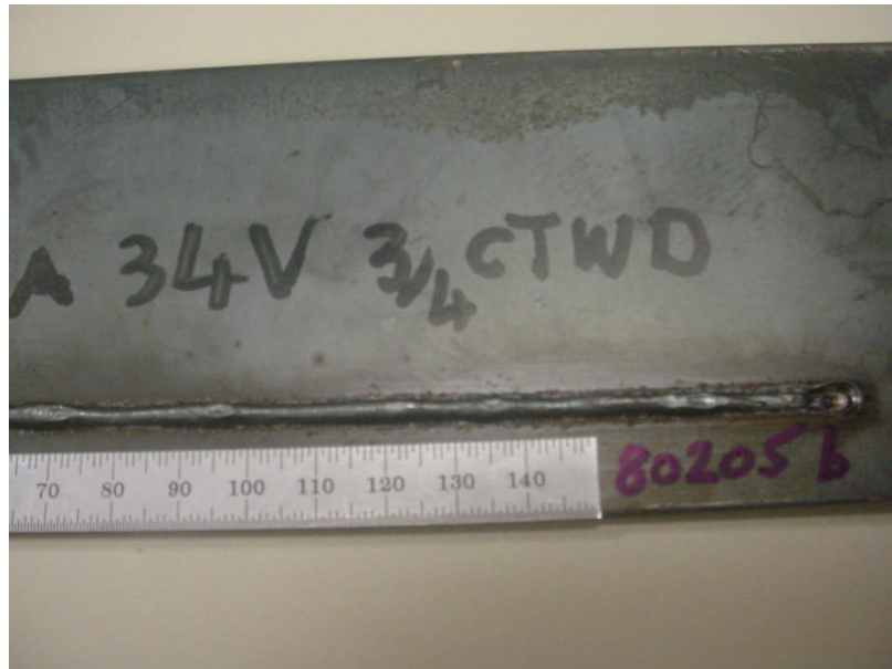
Figure 6.81 Plan View of GMAW-P BOP Humping and Weld Pool Cavity for Specimen 80205b WFS 15.2 m/min, TS 2.5 m/min, 225 A, 34 V, 19-mm CTWD, 1.6-mm Sheet
