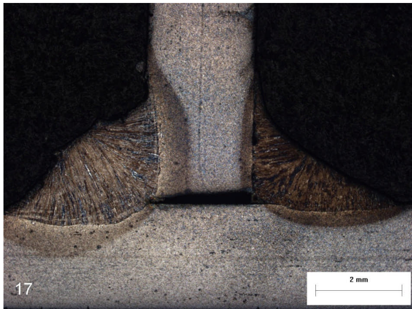
Figure 6.63 Macrosection (on left – tack on right) for a Single-Spot CO 2 LBW/GMAW-P Hybrid Weld made with 3.5-kW Laser Power at 3.0 m/min on 2-mm Sheet
