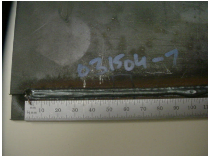
Figure 7.4 36-mm-Long Weld Pool with 3-mm Bead Width (12:1) Using Single-Spot 4-kW Nd:YAG/GMAW-P Hybrid on a Lap Joint
