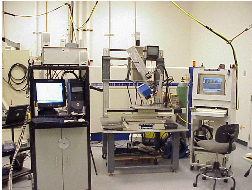
Figure 4.9 CNC Nd:YAG/GMAW-P Setup for PFO Evaluation, Including HSV, DAQ, and LASEdit Laser Programmer/Controller
