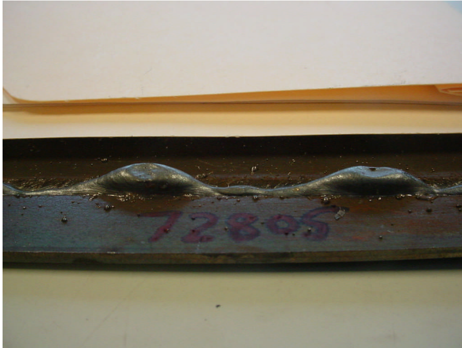
Figure 7.17 Side View of GMAW-P BOP Humping for 2.4-mm Sheet Specimen 72805
