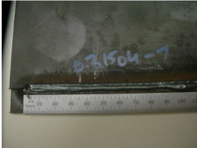
Figure 7.16 36-mm-Long Weld Pool with 3-mm Bead Width (12:1) Using Single-Spot 4-kW Nd:YAG/GMAW-P Hybrid on a Lap Joint
