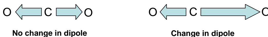
Figure 2-3: Change in the dipole moment of a molecule. The symmetric stretch in carbon dioxide is not IR active because there is not change in the dipole moment. The asymmetric stretch is IR active due to a change in dipole moment.
