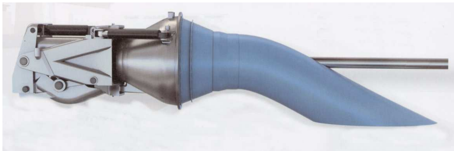
Figure 20: S type Jet Drive unit manufactured by Rolls Royce
