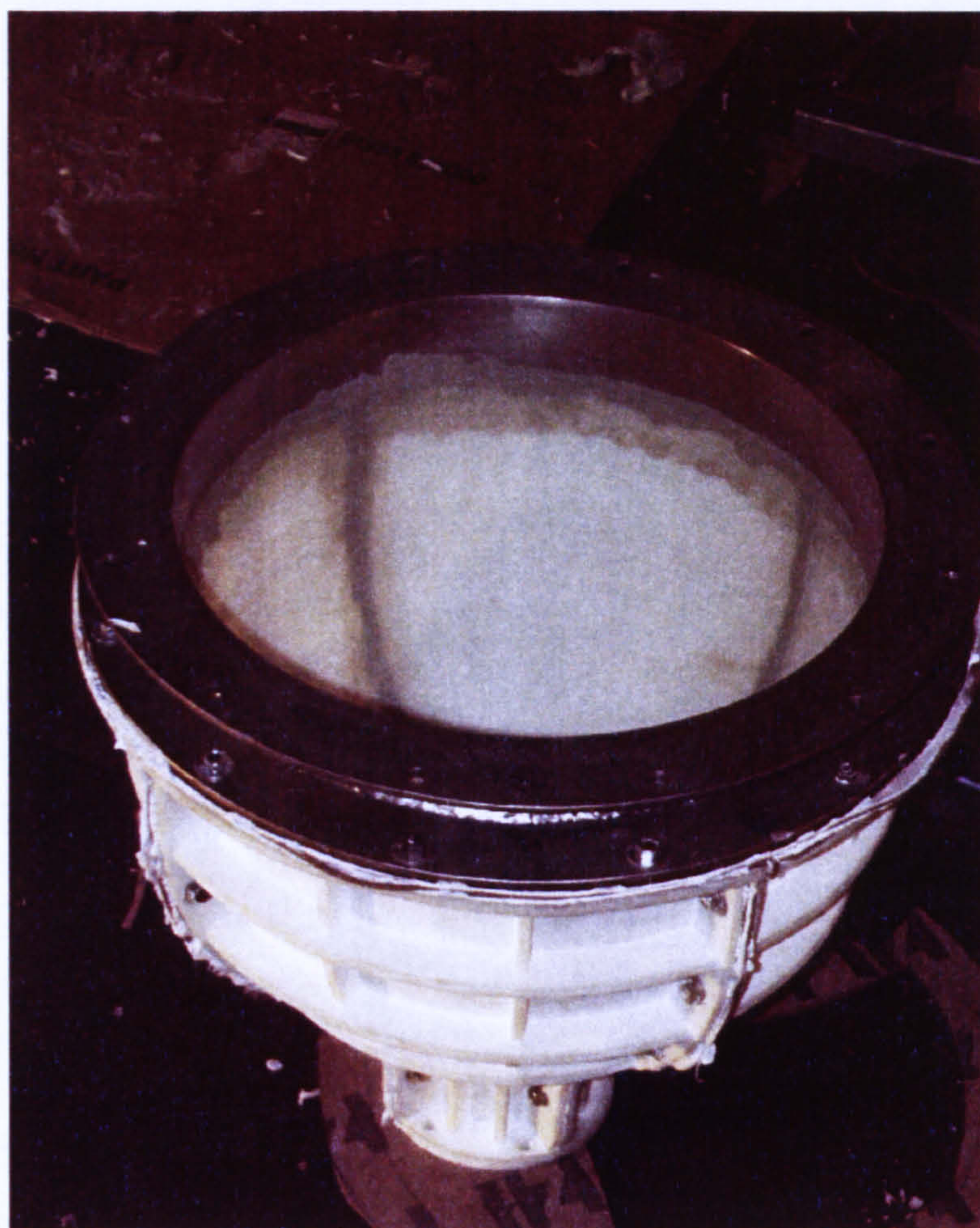
Figure 4.11: Assembly of the contraction sections and plenum spacer using cork seals, silicone sealant, and modelling putty. The photograph shows the four sections of the contraction with the seams filled by putty.
