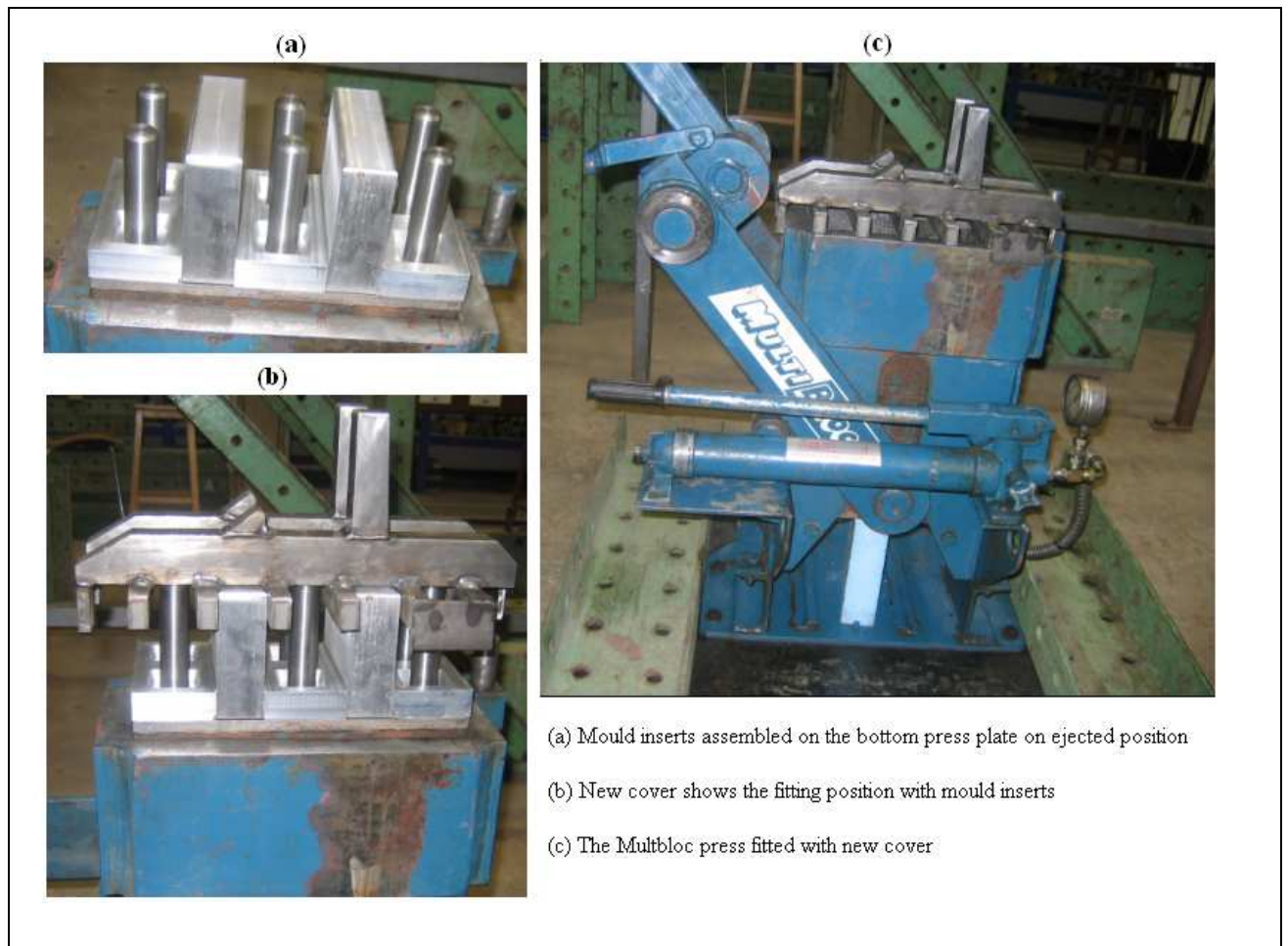
Figure 6.8 Multibloc press with new cover and moulding inserts
