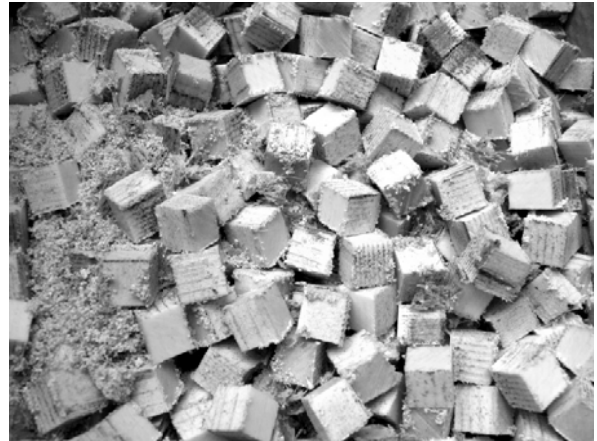
Figure 8.10: First downsizing of material pieces prior to grinding
