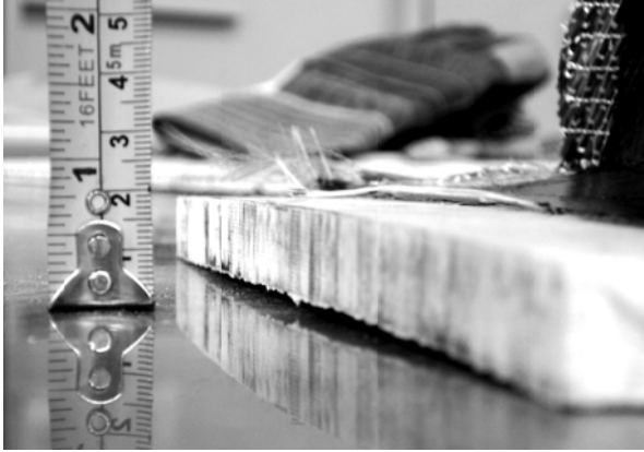
Figure 6.14: Warping in the substrate caused by asymmetrical bulk heating on thick laminates
