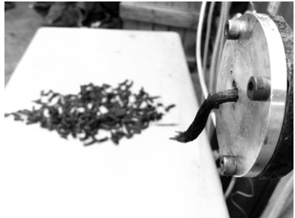
Figure 8.12: Compounding of the recyclate
