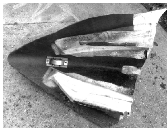
Figure 8.8: Bow section of the boat cut (sandwich internal structure in white over black hull)
