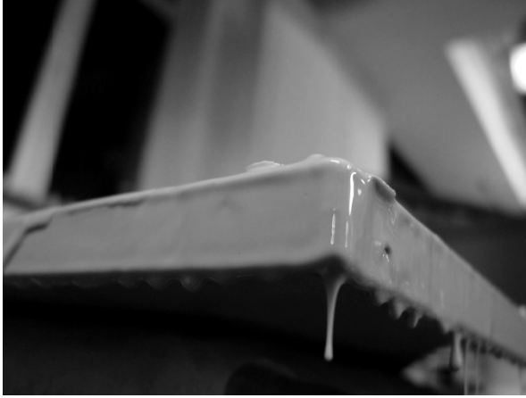
Figure 5.20: Flat, 15 mm tool being coated with P50 silicone rubber
