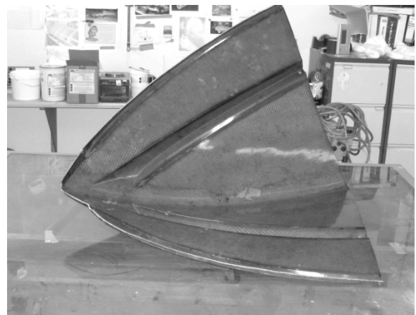
Figure 5.6: High temperature epoxy-glass test tool, shaped as a RIB bow
