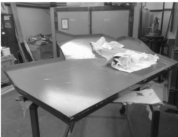
Figure 5.5: PTFE film coated 6 mm thick steel tool, for an experimental automotive part
