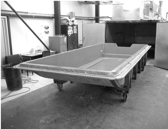
Figure 5.3: PTFE coated 15 mm thick steel tool used in BAE Systems for PP-glass military boats
