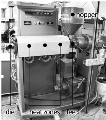
Figure 8.2: Single screw extruder
