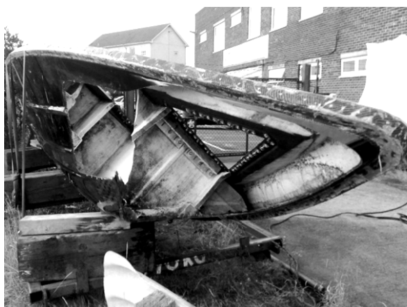
Figure 8.7: Hull opening on the Twintex® Atlantic 85 after material samples were cut out
