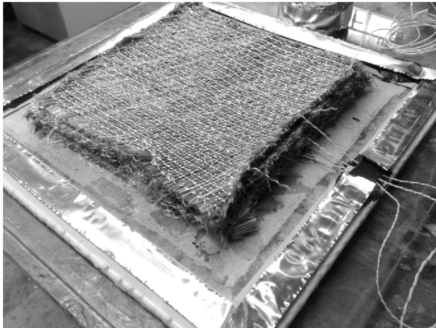
Figure 4.1: Ceramic tool with 6 layers of multi-axial Twintex ® and thermocouples for thermal measurements on bottom, middle and top layers
