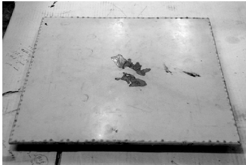
Figure 5.25: Tool state after 10 cycles, back surface (marks are remains of consumable adhesive tape used with thermocouples)
