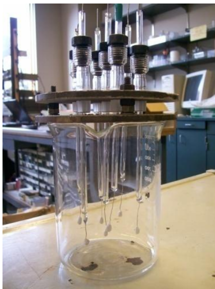
Figure 2.2. Preparation of the silver/silver chloride electrodes.
