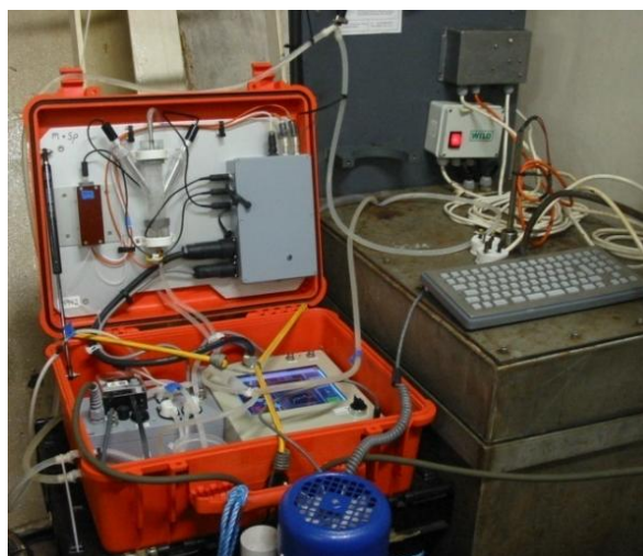
Figure 2.4. Drawing of the potentiometric pH system used in this study (top); and potentiometric pH system installed on the MV Pride of Bilbao (bottom). The grey lines on the drawing represent the data acquisition, the blue lines represent the solutions (seawater sample, buffer and liquid junction), and the green lines represent the valves and pump system.
