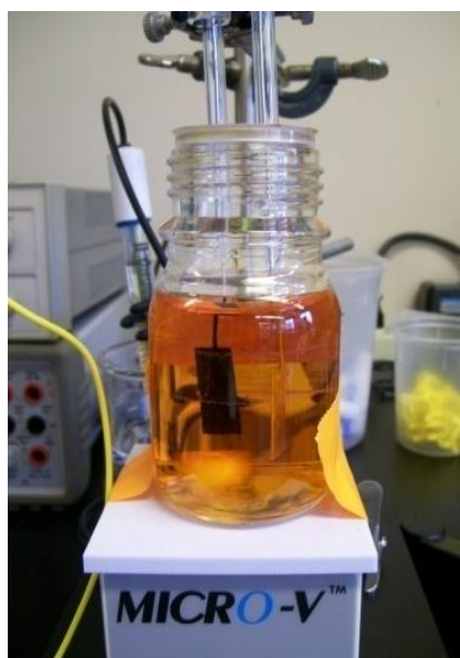
Figure 2.1. Platinization of the hydrogen electrodes.
