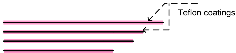
Figure 3.15 Teflon coated needles cut to different lengths
