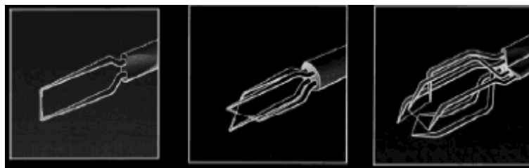
Figure 2.1 Hot film anemometry probes: one sensor, dual-sensor and three sensors respectively from left to right.
