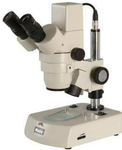
Figure 3.21 Digital stereo microscope MOTIC DM-143B used to measure the probe dimensions
