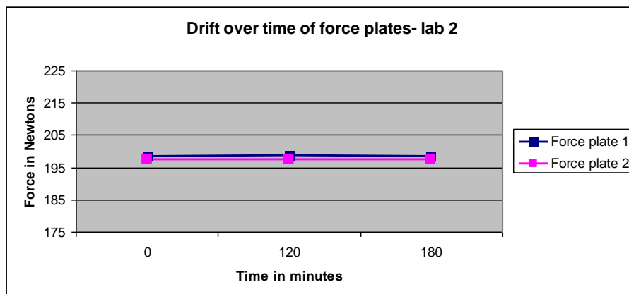
Figure 11.10 Graph showing drift in the data recorded by force plates in lab. 2 over three hours.
