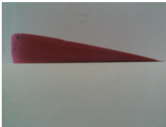
Figure 9.9 High density Ethyl Vinyl Acetate (EVA) wedge (12°) used in the project
