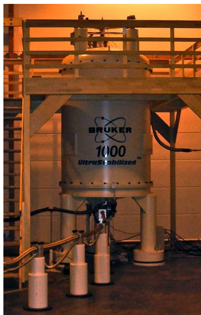
Figure 2.4. The world's first 1000 MHz NMR spectrometer installed at the Centre de RMN à Très Hauts Champs in Lyon, France.
