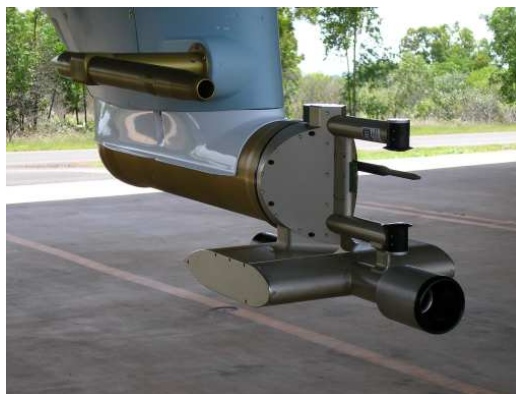
Figure 5.11: Port pylon of the Egrett. In the foreground is the CAS probe; to the rear and left (as viewed) is the aerosol inlet.
