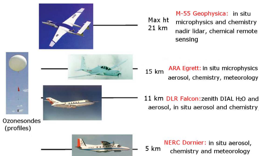
Figure 5.2: Montage of aircraft used in ACTIVE/SCOUT-O3 with a brief description of each. Figure from Vaughan et al. (2008).
