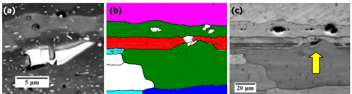
Fig. 6.8: Example of the PSN mechanism in the 0.4Mn alloy (3 min at 535°C): a) BSE image of a large constituent particle acting as a PSN nucleus as shown in the following pictures, b) EBSD texture map of the area containing the large particle of (a), and c) EBSD band contrast map of the same area. The position of the particle is pointed out by an arrow.
