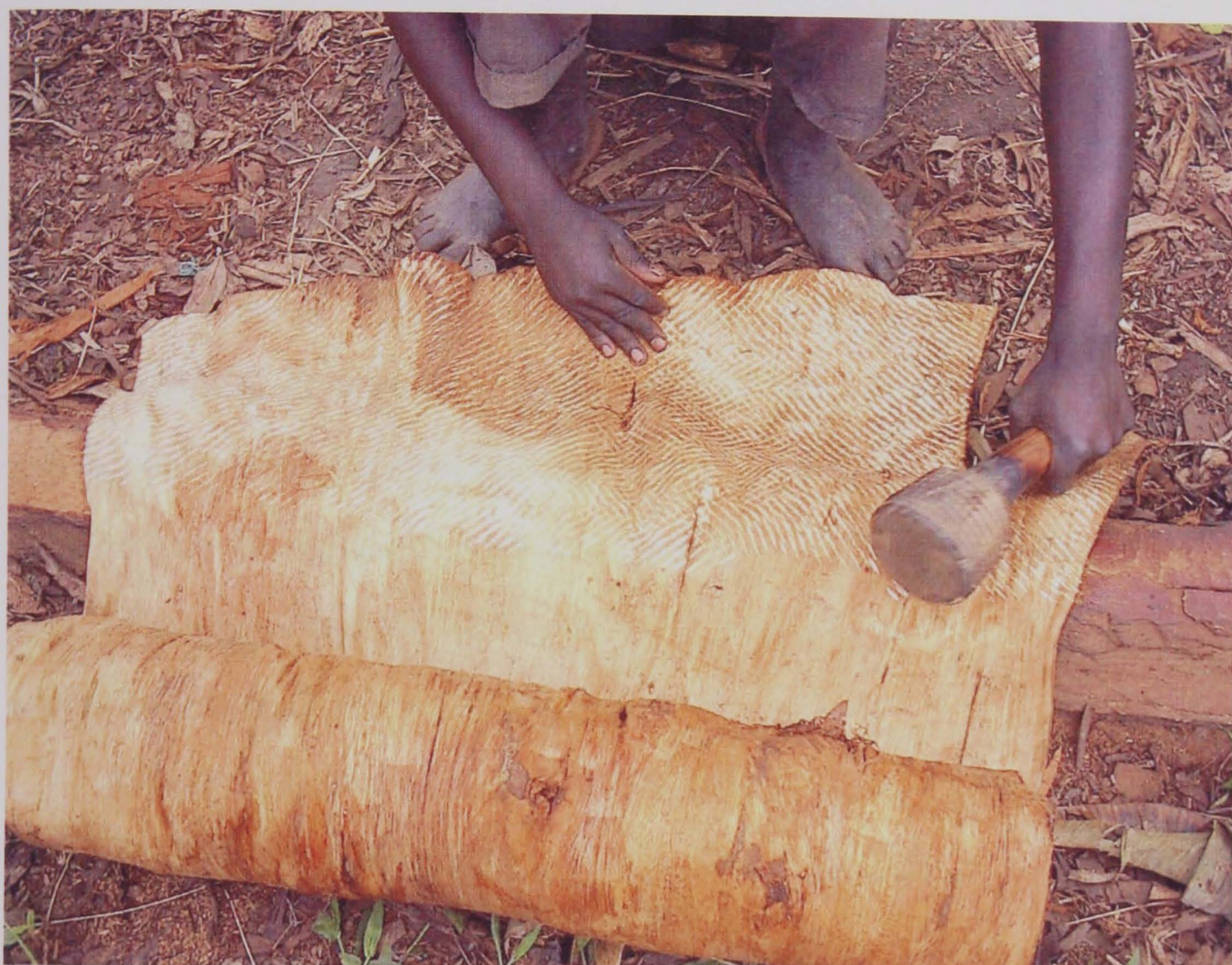
Plate 3.6 Initial diagonal beating to prevent the bark from splitting. Photo by the author
