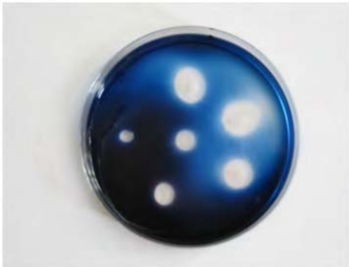
Figure 4-9 Residual amylase activity revealed using the RED assay. The smaller the halo the more thermal processing the amylase has received (100mm plate diameter)
