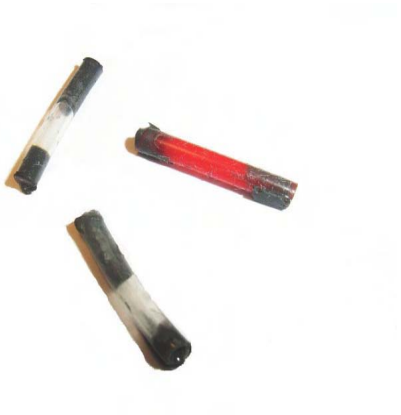
Figure 2-4 Capsule enzymatic TTIs (10mm length, 3mm tubing)
