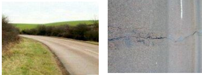
[Figure 5.7] Road surfaces used by Honda for their steering wheel vibration tests.
