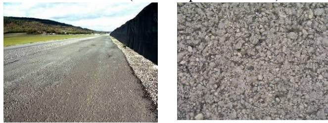
[Figure 5.4] Road surfaces used by Michelin for their steering wheel vibration tests.
