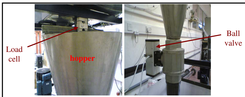
Figure 6-10: Photographs of the hopper load cell system
