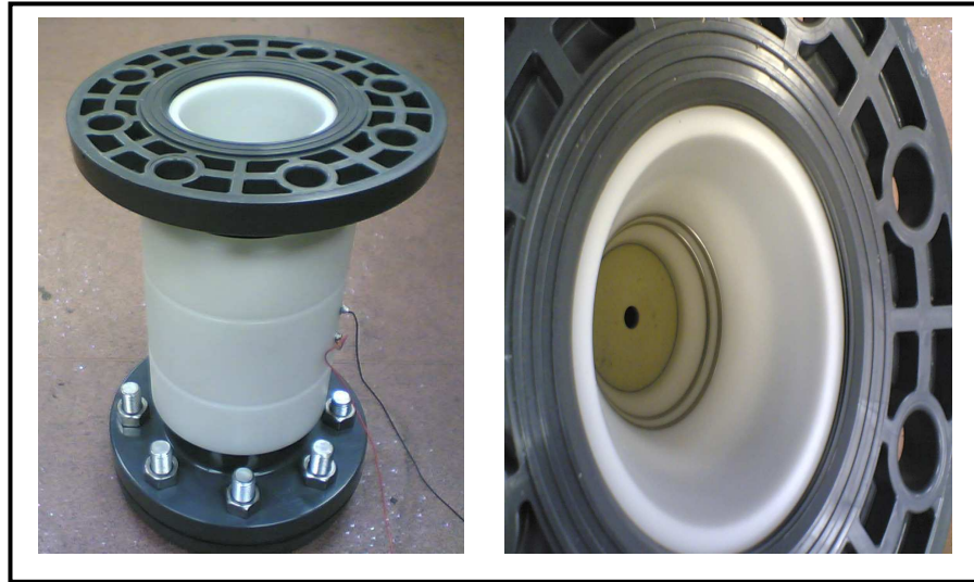
Figure 4-6: Photos of the conductance inlet void fraction meter (CIVFM)
