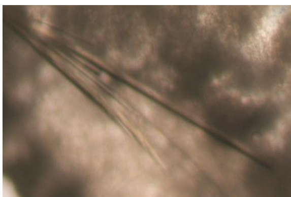
Figure 3.8 Crystals of the FAD/NADPH binding domain of MSR. The conditions used to produce this crystal are: one drop of enzyme sample (1 µL, 10 mg/mL) was mixed with 1 µL mother liquor (0.1 M Tris/HCl, pH 7.5, 0.2 M KBr), and incubated with 98 µL the same mother liquor in a reservoir at 19 °C. Crystals formed after about 4 days.
