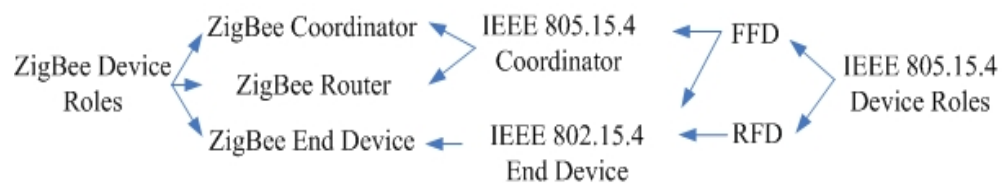
Figure 4.5 - Device Roles in the IEEE 802.15.4 and ZigBee Standard
