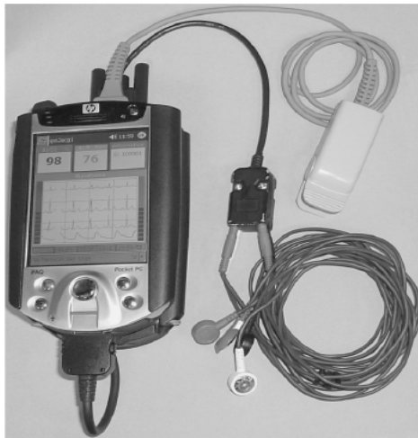
Figure 2.3 - A Wireless PDA-based monitor (Lin et al. 2005)
