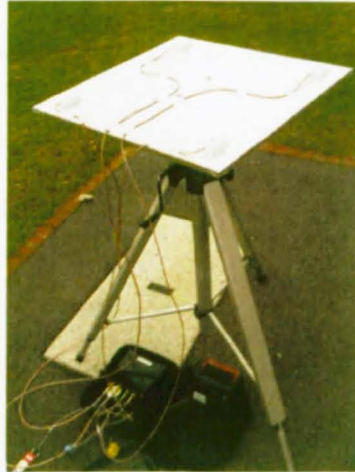
Figure 7-7 Close-up of mock-up facet showing four GPS L1 patch antennas
