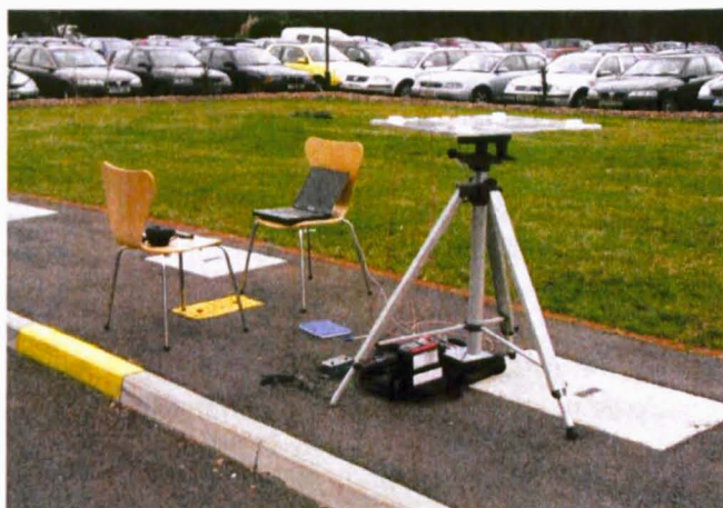
Figure 7-6 Testing GPS attitude code using a mock-up satellite facet
