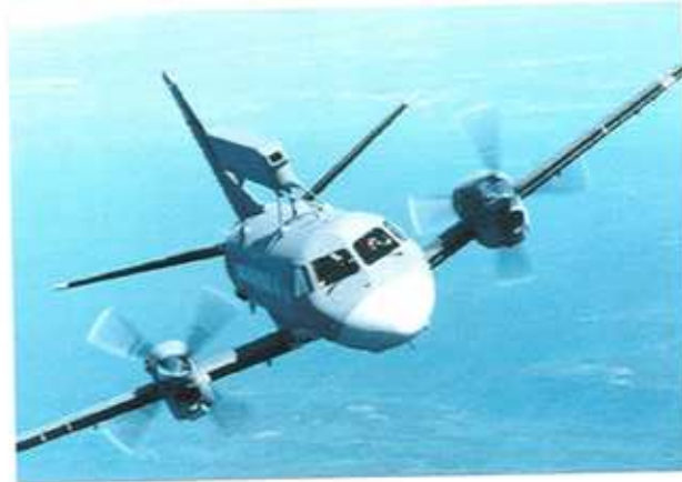
Figure 1.2: Erieye is a long range pulse Doppler radar, fitted with fixed active phased array antenna [17].
