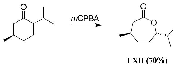
Scheme 1.37. Synthesis of (-)-menthede ( LXII ) prepared from (-)-menthone. (overall yield from (-)-menthone in parentheses).
