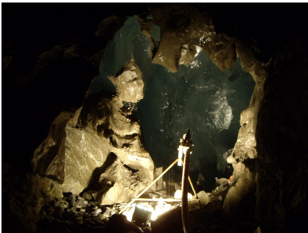
Hose used in hot water drilling of the ice cave and the ice cave which allows for access to pristine subglacial samples. The hose support is about 90 cm high, November 2008.
