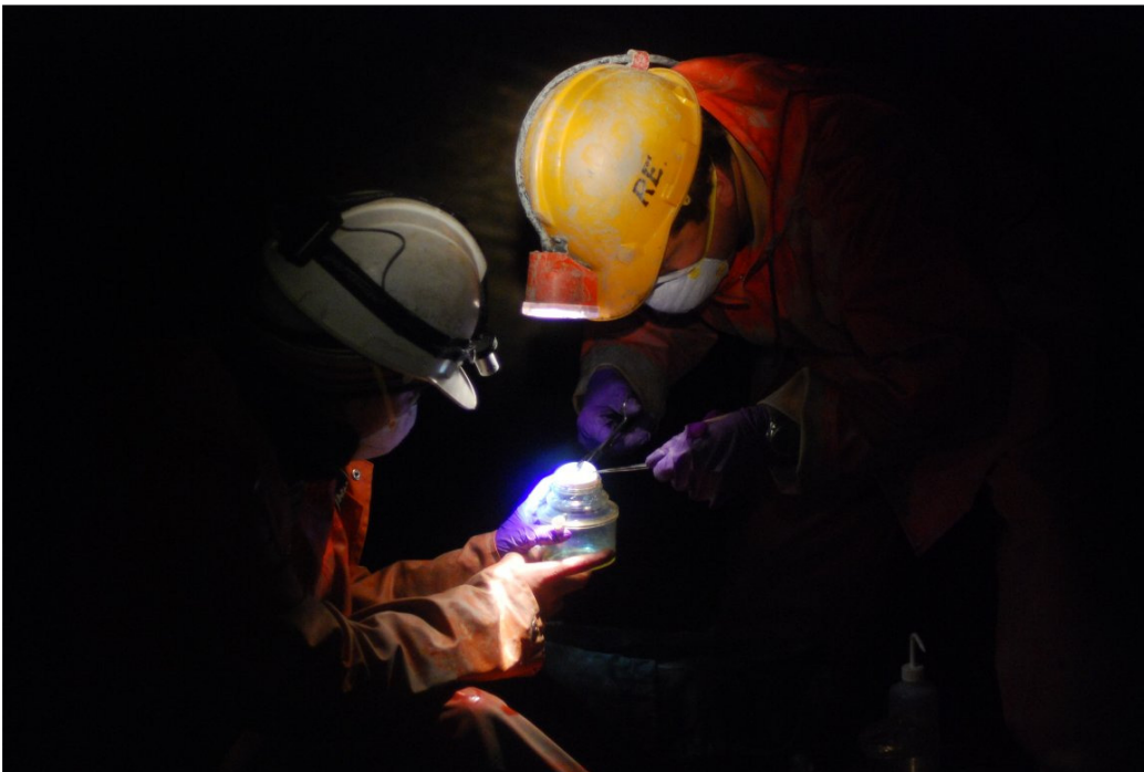
Sample preparation in the tunnel system. Samples were filtered and the membranes split in the tunnel and then transported back to the satellite laboratory to conduct analysis, March 2009.
