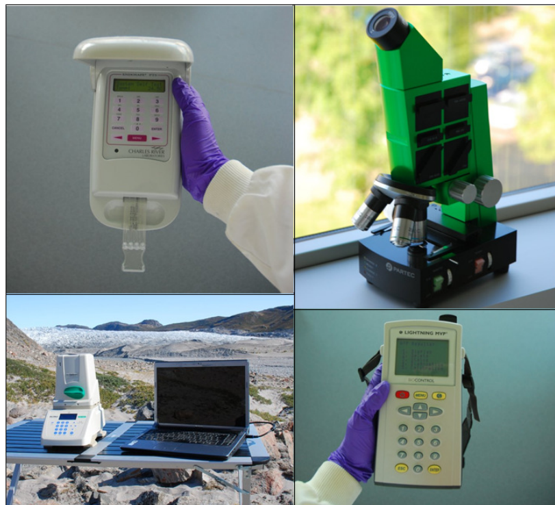
Figure 2-2. Field portable microbiological life detection technology. Starting in top left and moving clockwise: Endosafe ® -PTS ™ with cartridge (Charles River Laboratories International Inc., MA, USA), CyScope ® (Partec GmbH, Germany), LIGHTNING MPV ® (BioControl Systems Inc., WA, USA) and MiniOpticon ™ (Bio-Rad Laboratories, CA, USA).
