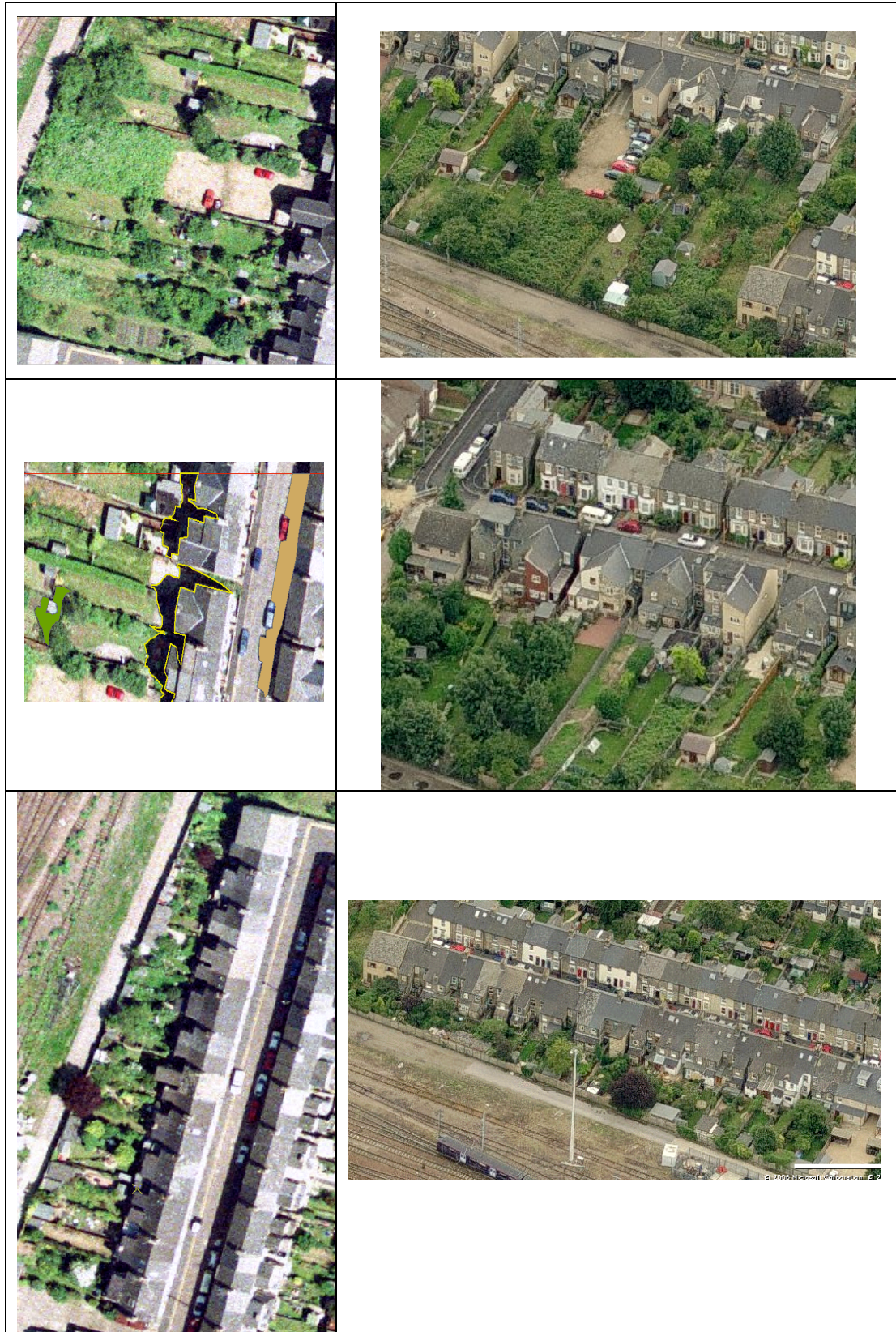
Figure 6-31. Examples of the sealed surfaces that are in shadow in a true colour aerial photo (left column) and their identification with the use of an oblique image (right column)
