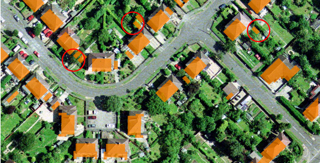
Figure 7-5 Misclassification results due to relief displacement between EO and ancillary data as well as not updated thematic information ancillary data (in red circles)
