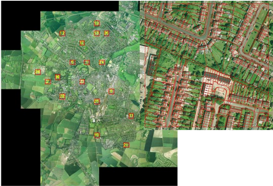
Figure 4-1 Orthophoto mosaic of the aerial photography of Cambridge with the 250 x 250 m 18 sample areas within the city of Cambridge. The example square illustrates the detail of the 1:1250 scale Ordnance Survey Master Map.
