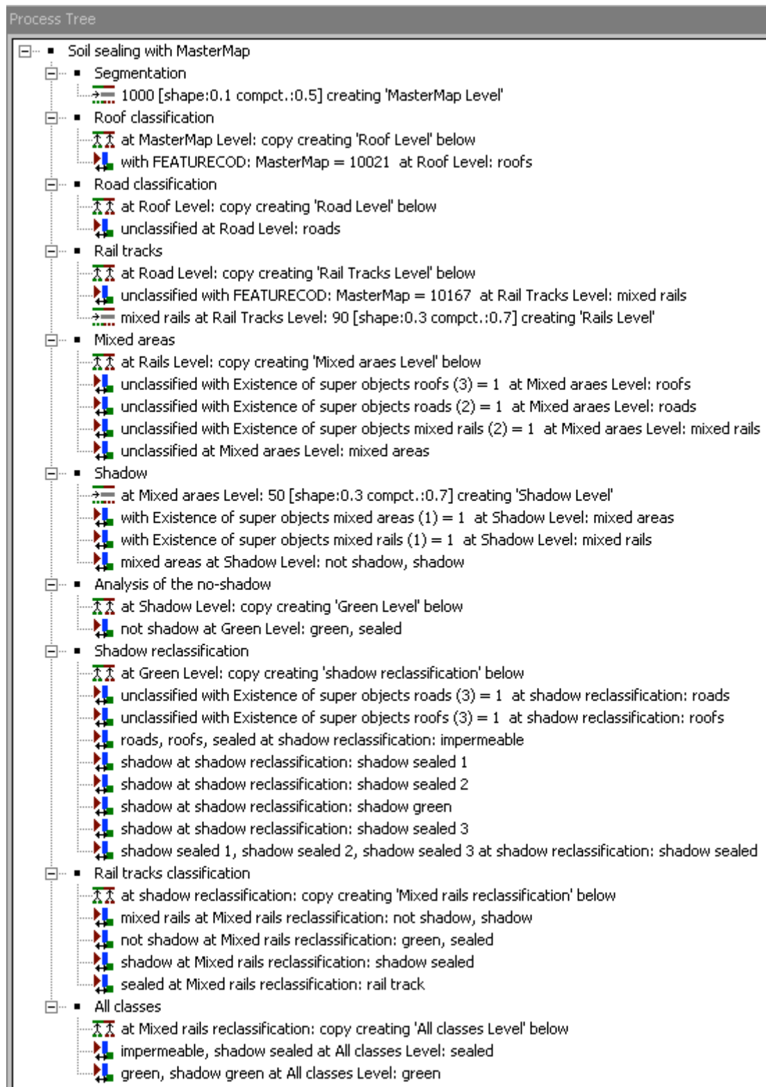
Figure 7-1 The complete rule-set, using processes in eCognition, for the development of the object-based model
