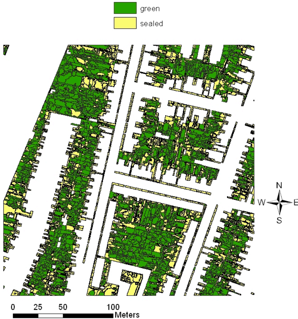
Figure 7-4 The automated rule-based classification results after masking out the OS Mastermap polygons
