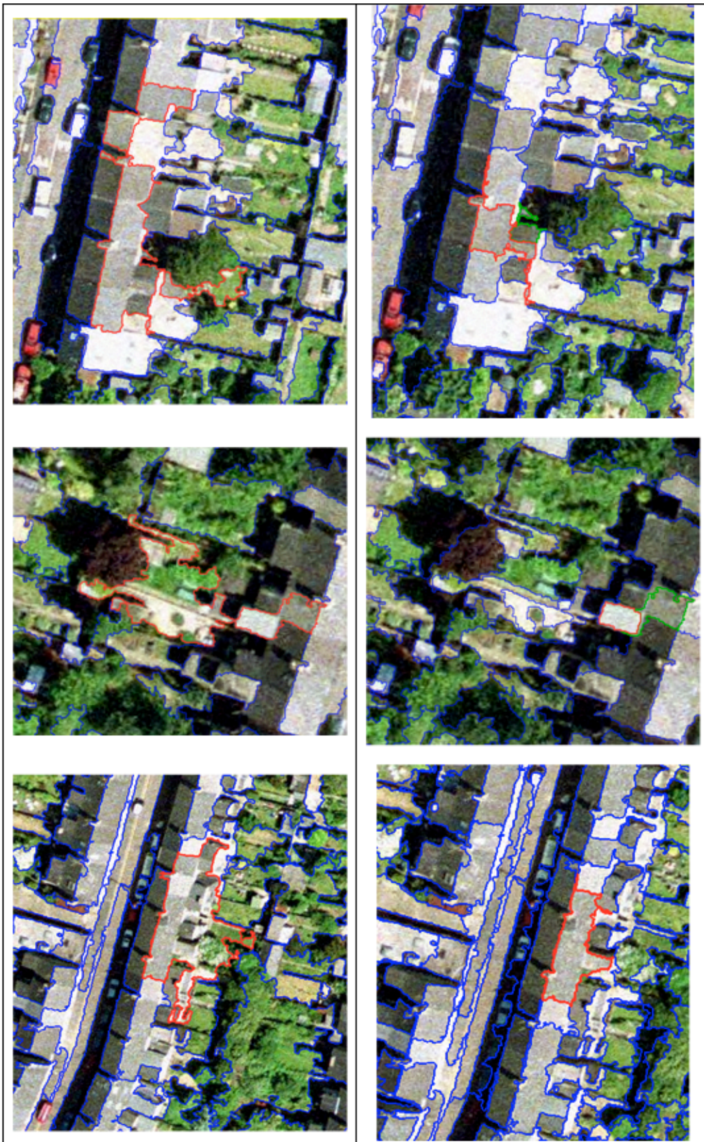
Figure 6-21 Examples of the segmentation results when using scale-225 (left column) and scale 90 (right column)
