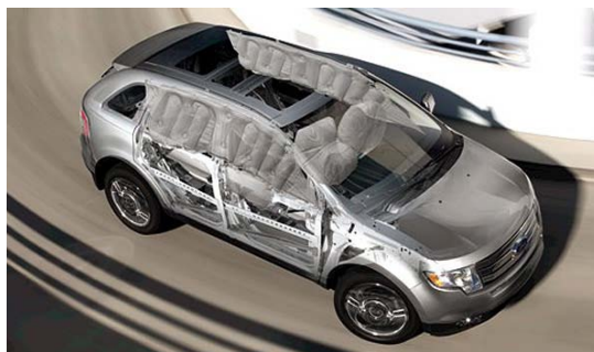
Figure 3.4 Ford's Safety Canopy system deployed on the Ford Edge (From: www.fordvehicles.com/crossovers/edge/features/interior , accessed 15.6.09)
