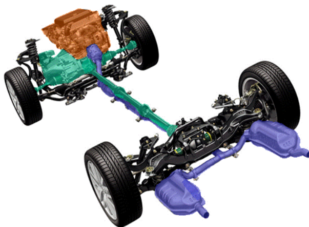
Figure 5.20 ICE Power train schematic
