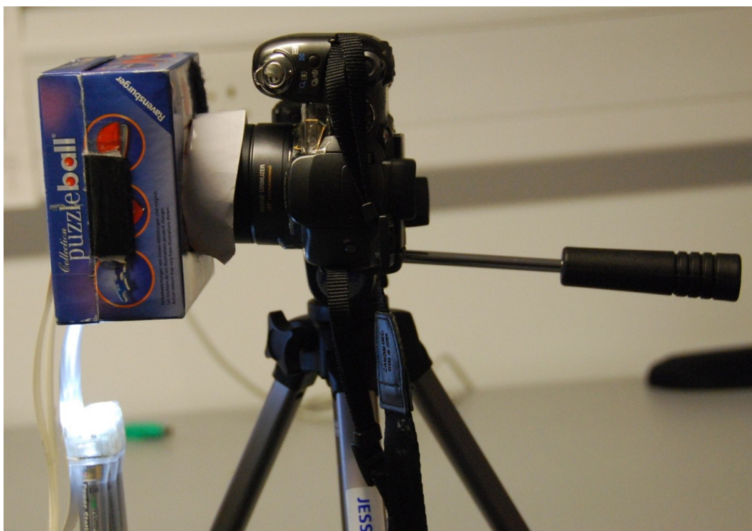
Colour plate 5.4 Dark chamber with attached camera and the light source underneath.
