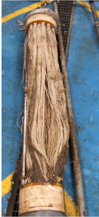
Figure 7-26 – Membrane after dosing trials had been carried out.
