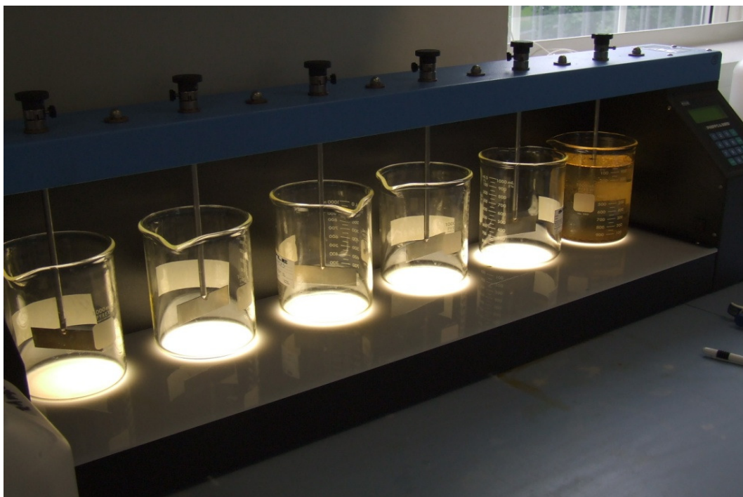
Figure 4-12 – Jar tester used for the ancillary chemical investigation.
