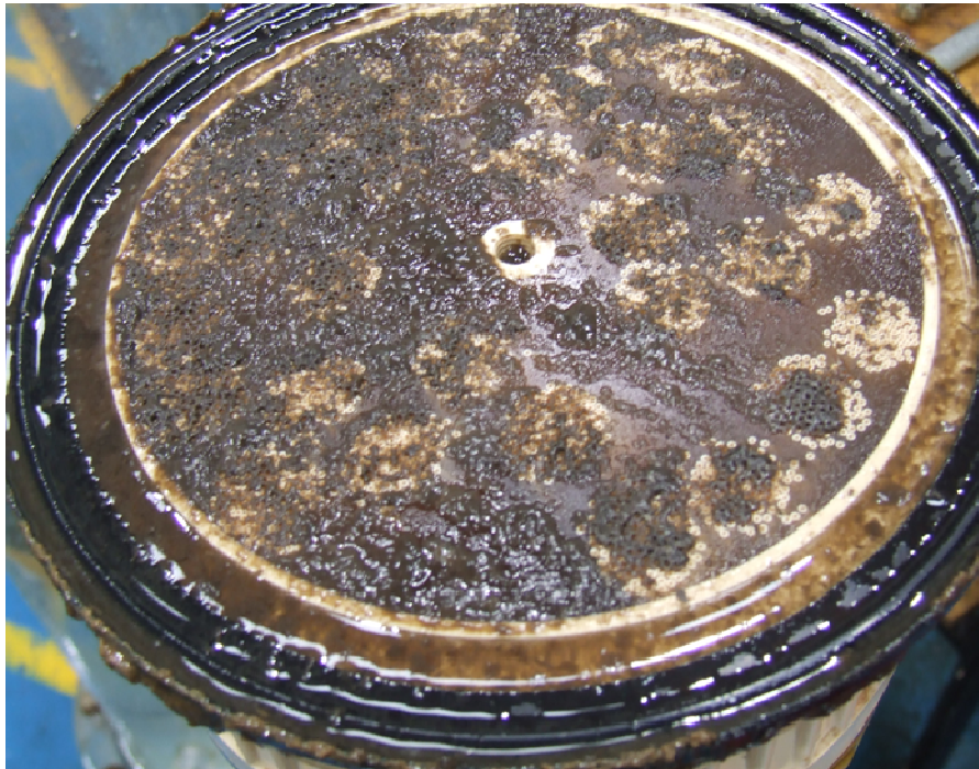
Figure 7-4 – Biomass ingress into the permeate side of the membrane.
