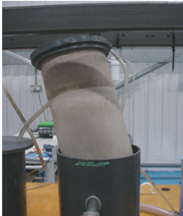
Figure 4-4 – Photograph of a porous pot showing the membrane liner.
