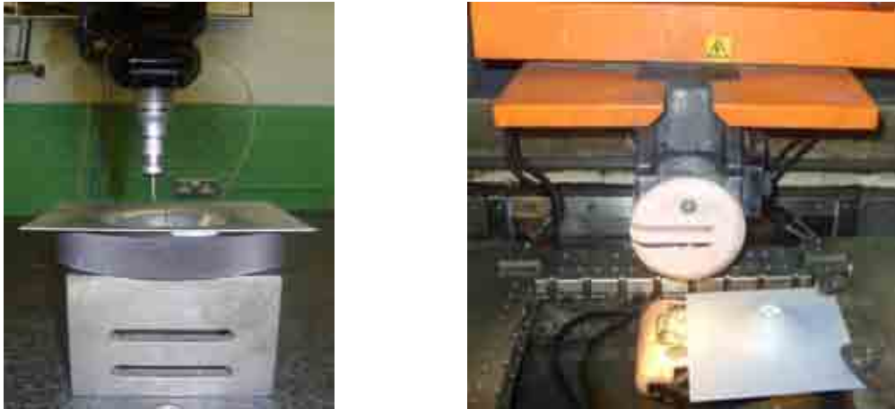
Figure 5.2: (a) The profile measuring setup, (b) the cutting process for the truncated cone along the central plane.
