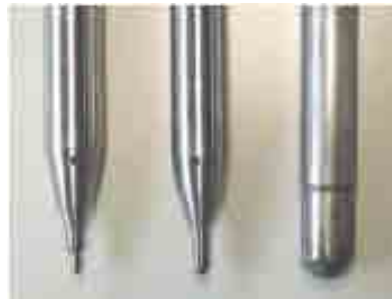
Figure 2.17: Cemented carbide tools with diameters of 6, 10 and 30mm [73].
