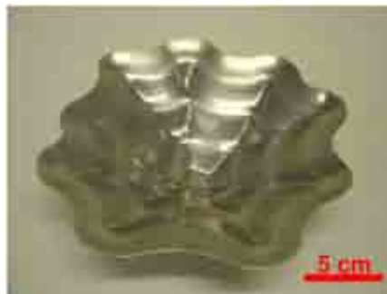
Figure 2.22: A bespoke light shade manufactured by AISF and designed by Rachel Tomlinson, University of Cambridge in 2005. The striated surface is a desirable feature of the product.
