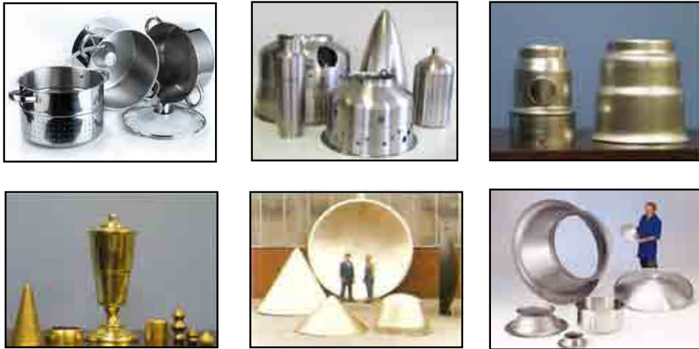
Figure 2.3: A wide range of products can be produced by conventional spinning [10-12].
