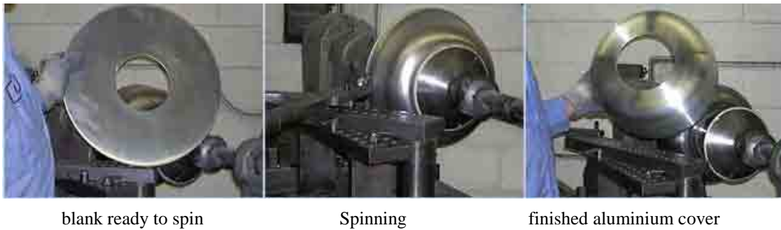
Figure 2.5: A spinning process [14].
