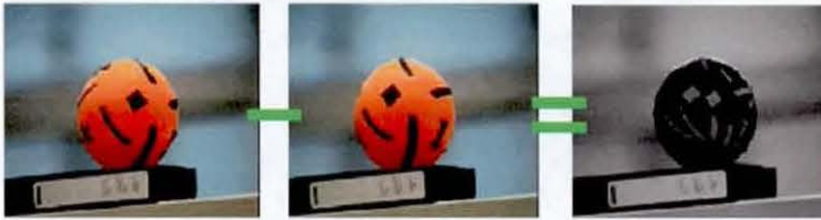
Figure 3-14: Difference between two acquired images, adapted from (Tamaki et al. 2004)
