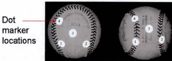
Figure 3-4: Dots for spin measurement, adapted from (Alaways and Hubbard 2001).
