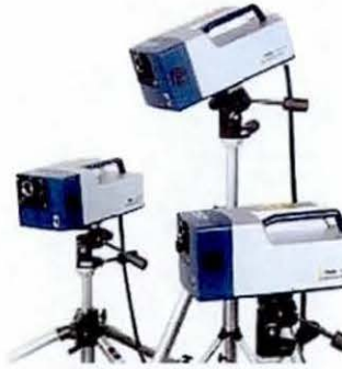
Figure 2-29: PSV-400-3D system, three individual scanning heads.
