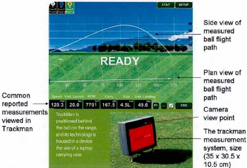
Figure 3-8: The Trackman system, adapted from (Stachura 2006).
