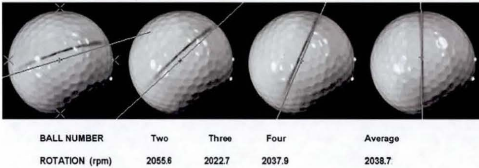
Figure 4-6: Flightpath analysis of spin rate, using golf ball collage.
