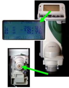
Figure. 2.5: The Konica Minolta hand held spectrophotometer CM5031 used to quantitatively measure the colour of harvested broccoli genotypes and colour change during storage.
