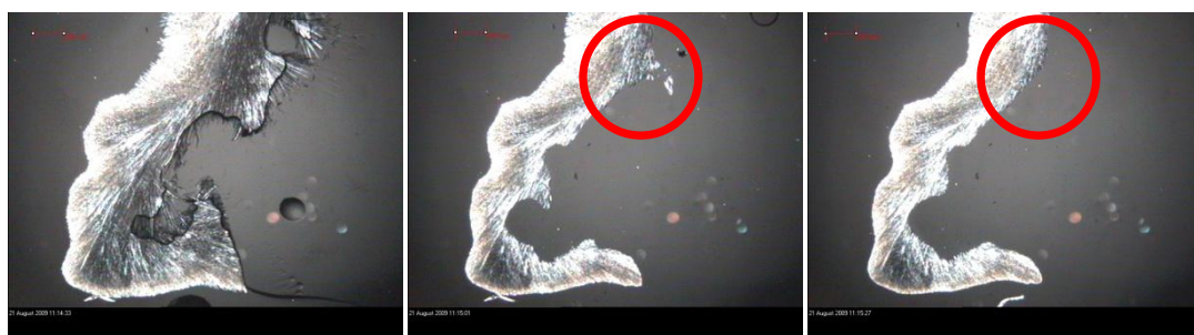
FIGURE 53- THE EFFECT OF CONTINUED ADDITION OF ACETONE ON THE CRYSTALLINE PRECIPITATE OF 2:1 SALT FROM ACETONE USE AS AN ANTI-SOLVENT.
