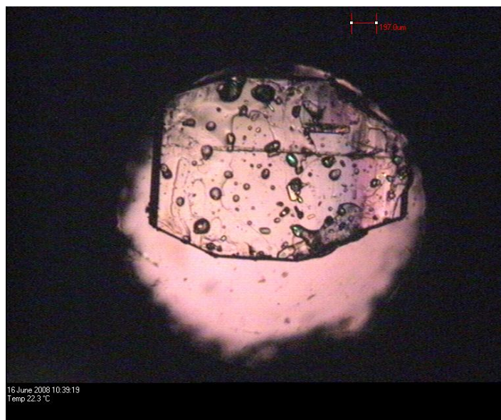
FIGURE 54- IMAGES OF 1:1 EPHEDRINE PIMELATE CRYSTALS GROWN FROM WATER
