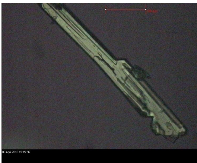
FIGURE 94- CRYSTAL FORMED FROM EPHEDRINE AND BENZOIC ACID IN WATER
