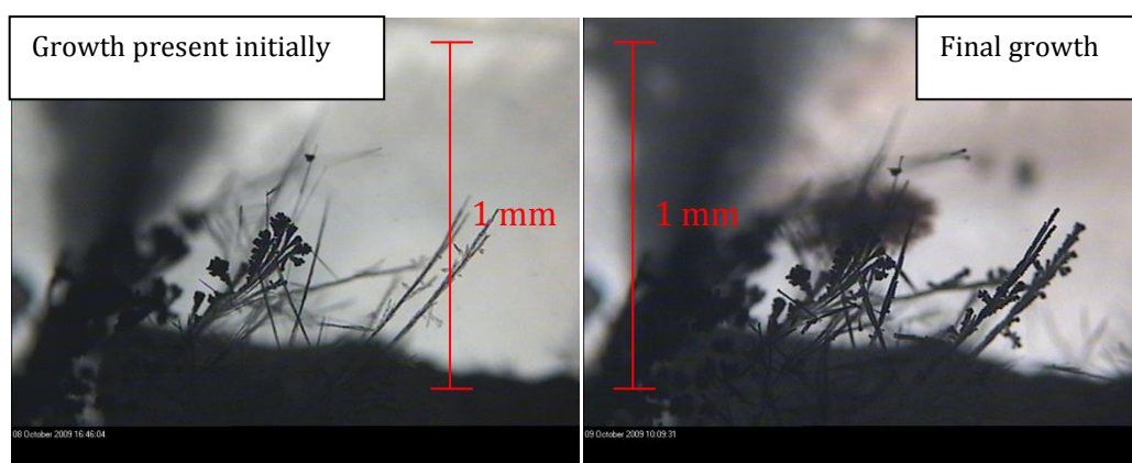
FIGURE 80- MICROSCOPE IMAGES OF NEW PRODUCT GROWTH FROM CONTACT OF EPHEDRINE AND BENZOIC ACID AT ROOM TEMPERATURE. IMAGES RECORDED OVER ONE DAY.
