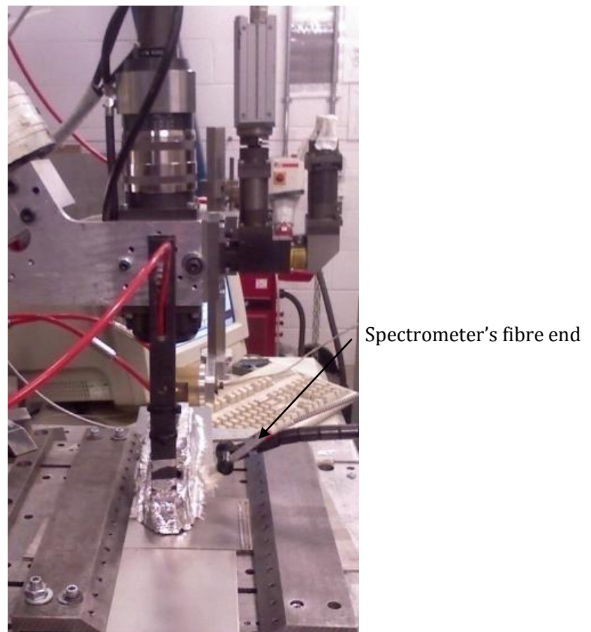
Figure 4-8. Typical configuration/position of the spectrometer's optical fibre end.
