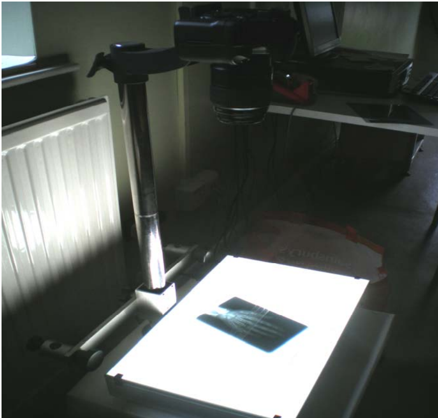
Figure 6.1: Photograph of setup used to digitise radiographs, optimised for measurement of MI.
