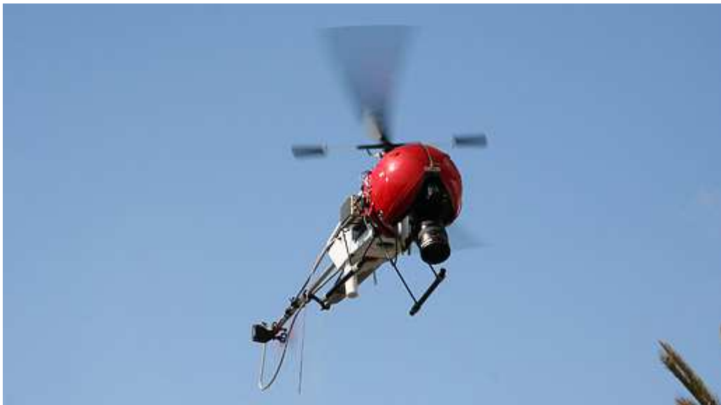
Figure.4. 27 Camera embedded on an UAV
