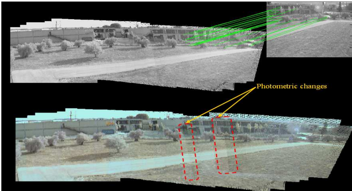
Figure.4. 33 Image mosaic from a set of image acquired by a camera embedded on an UAV
