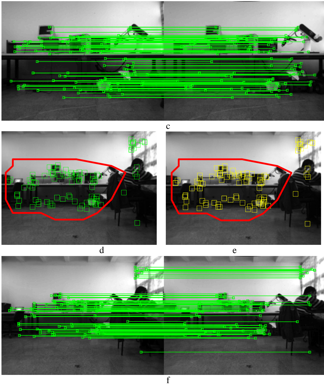
Figure 6. 9 Feature extraction and matching, a, b) features extracted in left and right image observed by robot1, c) Features correspondence for robot1; d,e) features extracted in left and right image observed by robot2, f) Feature correspondence for robot2, shared region observed by robot 1 and 2 are limited by the red line.
