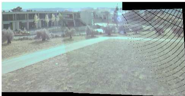
Figure.4. 36 Image after photometric registration (the intensity change is almost removed)
