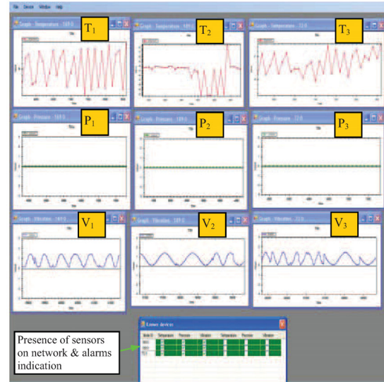
Fig. 8. Screen shot from monitoring software for 3 sensor nodes monitoring temperature, pressure and vibration
