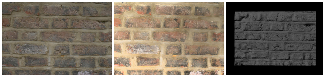
(a) Original Image of the material under diffuse lighting conditions. (b) Recovered albedo map. (c) Recovered meso-structure.
