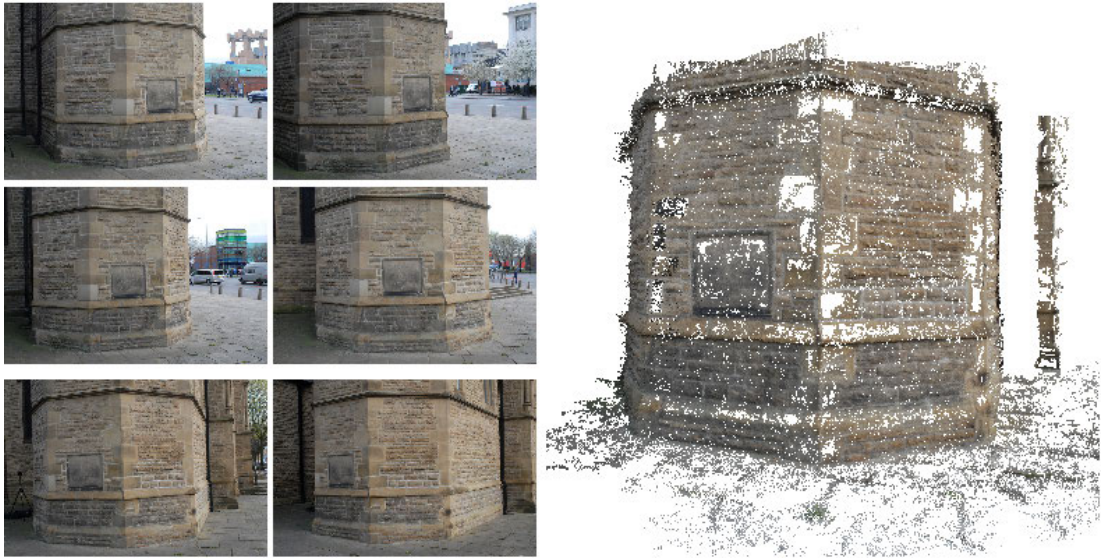
Figure 2.1: Sequence of multi-view photographs used for reconstruction and resulting point cloud.
