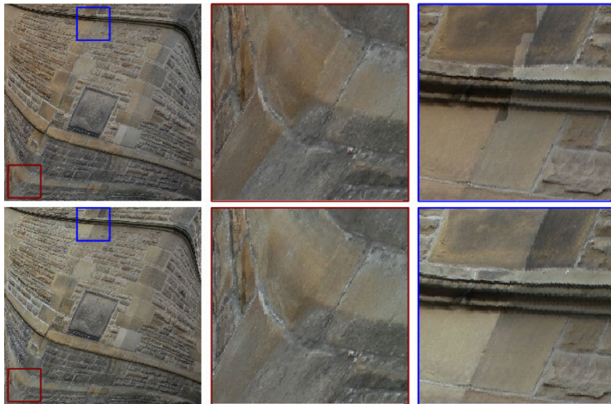
Figure 5.4: Remaining seams due to lighting variation shown in the top row, can be totally removed using poisson reintegration as can be observed in the bottom row. The middle and right columns correspond respectively to the areas inside the red and blue squares highlighted in the right column images.
