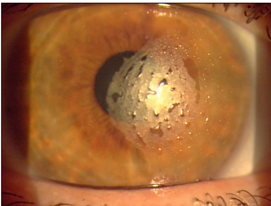
Figure 4.8: A non-wetting and heavily deposited region on an air-cured contact lens after 10 minutes of wear.
