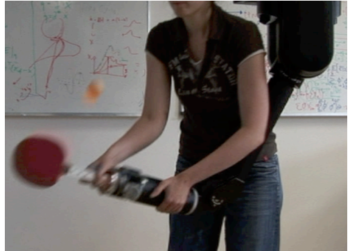
Figure 5.3: Data collection was performed using a Barrett WAM robot as haptic input device.
