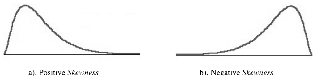
Figure 5.18: Diagrams used to illustrate positive and negative Skewness
