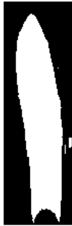
Figure 5-34: The binary image of flame with no excitation
