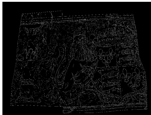
Figure 5.3.7 Result of Canny edge detection on image of front of Lion tapestry in CIELAB colour space with specified threshold and standard deviation values
