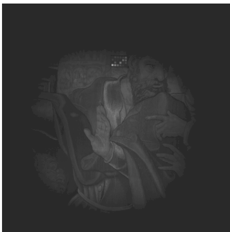
Figure 4.3.11 540 nm wavelength band hyperspectral image showing the circular area produced by the filter. Note the Mini ColorChecker chart in the periphery
