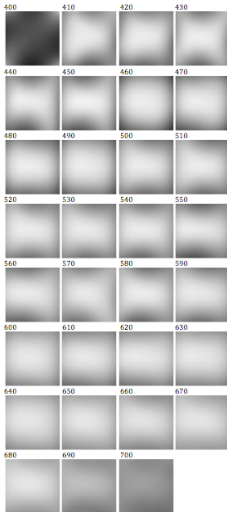
Figure 4.3.26 Cropped hyperspectral images of a white card showing the central 50 cm by 50 cm area
