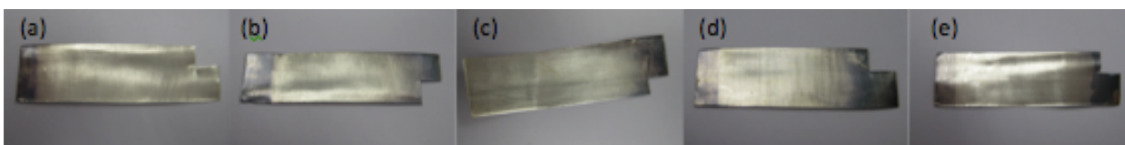
Figure 3.3.31 Thermal aged silver coupons. One sample from each of the 5 levels of the visual corrosion scale; (a) W Copper (1), (b) W Woad (2), (c) W Oakgall (3), (d) W Coch (4), (e) W Madder2 (5)
