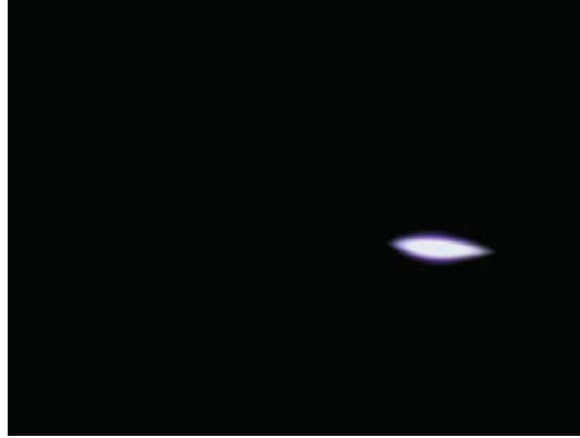
Figure 6.1: Plasma in air observed with top-view CCD camera. The length of the filament, obtained by 100\times MO when E \cong 15\mu\text{J} , is about 20\ \mu\text{m} .
