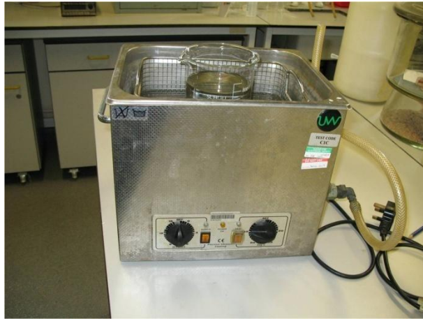
Figure 5-5 Ultrasonic cleaning bath, 30 kHz, 60W.
