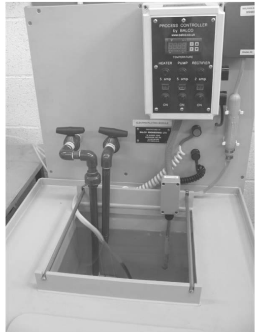
(b) Electroplating tank set-up
