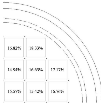
Figure 4-44 Pattern scale uniformity distribution of DC( 10 \text{ mA/cm}^2 ) electroplated indium bumps on a quarter of the 4 inch wafer pattern with a thief ring design.
