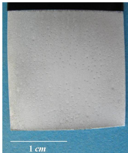
Figure 3-6 ‘Pitting’ effect observed on the surface of electroplated indium caused by the hydrogen bubble evolution when the peak current density i_p = 300 \text{ mA/cm}^2 .
