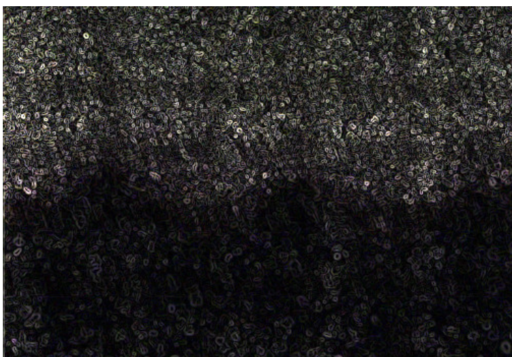
Figure 3.14 Image of ceramic platinum ink (top half) and ceramic substrate (bottom half) after application of the Sobel edge detection algorithm in ImageJ
