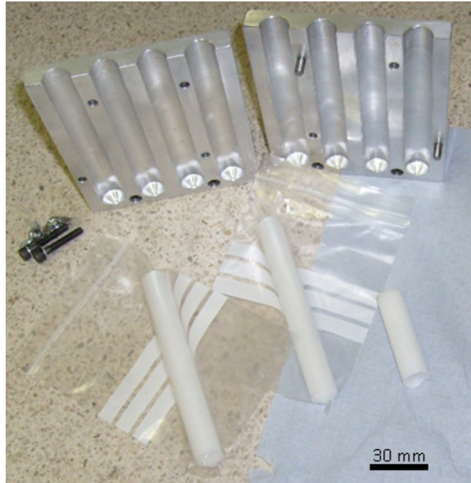
Figure 3-11 Cartridges of the jetting materials
