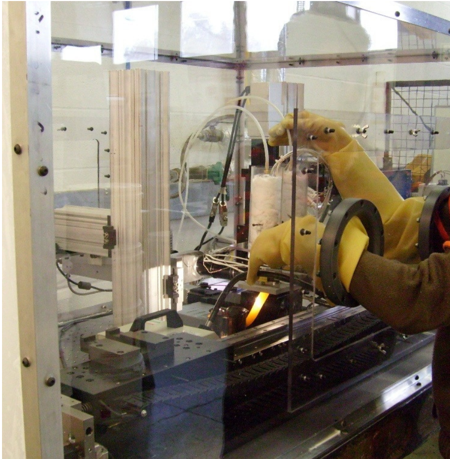
Figure 3-20 Glove box to control process environment
