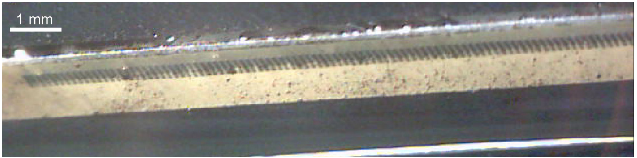
Figure 5-3 Black particles in the thin molten layer on the nozzle plate with a vacuum level of 20 mbar
