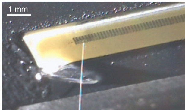
Figure 5-4 Single jet of caprolactam (17.5 V, 4 kHz, 15 mbar, Set 2)
