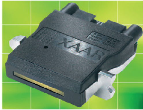
Figure 3-2 Printhead Xaar 126/80 (Xaar plc 2008)
