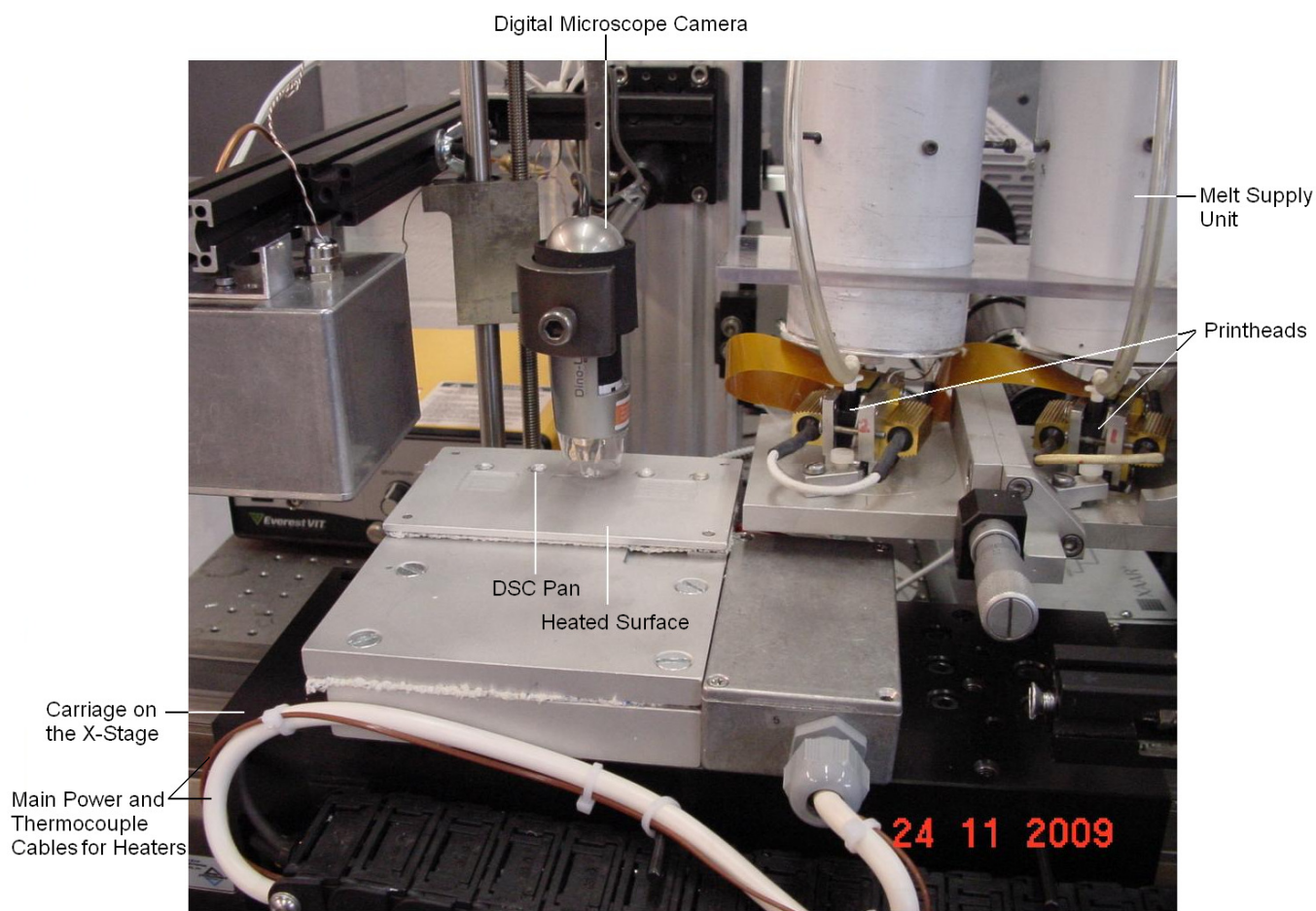
Figure 3-18 Heated substrate on the X stage carriage for deposition into DSC pans
