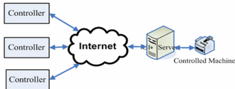
Figure 3. 2 Many-to-One Remote Control Architecture
