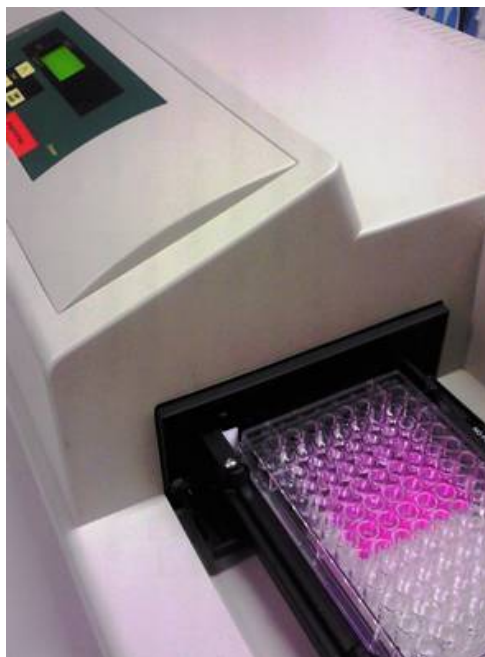
Figure 2.4 | SRB-stained cell protein aggregates in a 96 well plate reader. Cells were seeded at ascending densities to establish the optimum density for the cytotoxicity assays using the renal carcinoma cell lines
