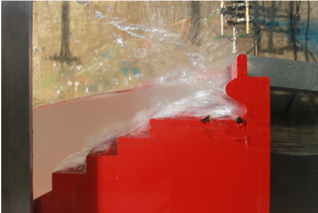
Figure 7.12: Uprushing water on the seawall, showing eddies at steps and splashing from recurve wall
